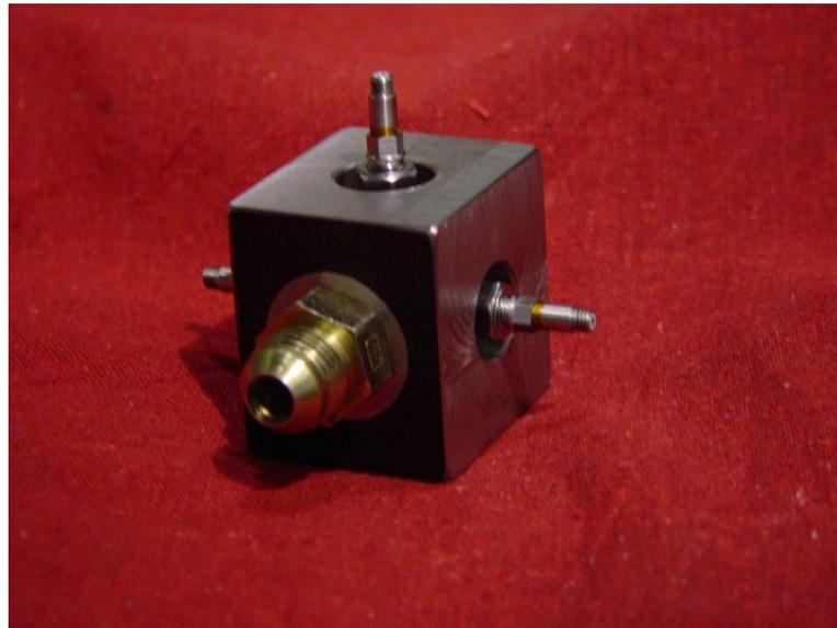
**Figure 5-11: Picture of calibration block with three sensors installed.**
