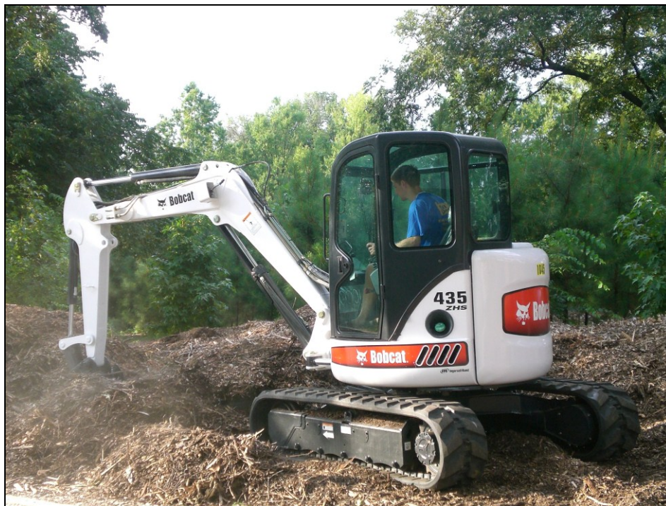
Fig. 4. Bobcat 435 mini-excavator in a normal dig cycle
