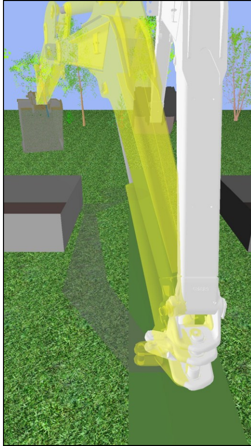
Fig. 31. Ghost arm on the excavator simulator
