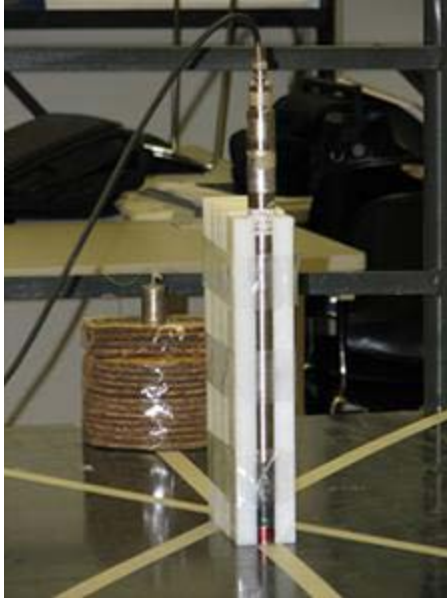
Fig. 7.6. ^3\text{He} detector inserted into the bare polyethylene parallelepiped (from an unrelated experiment).
