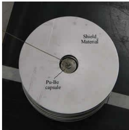
Fig. 6.7. Placement of the PuBe source into the nickel shield.
