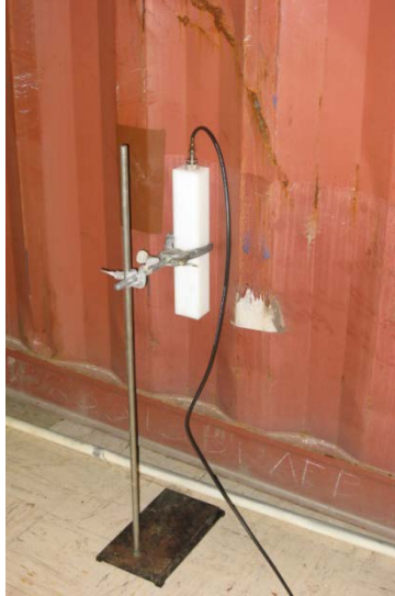
Fig. 7.9. Moderated detector assembly positioned against the CONEX container.
