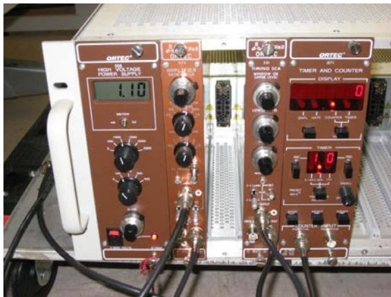
Fig. 7.2. NIM components for the ^3\text{He} and \text{BF}_3 systems.
