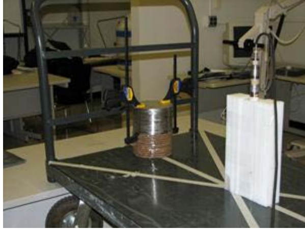
Fig. 6.8. PuBe source in its nickel shield.
