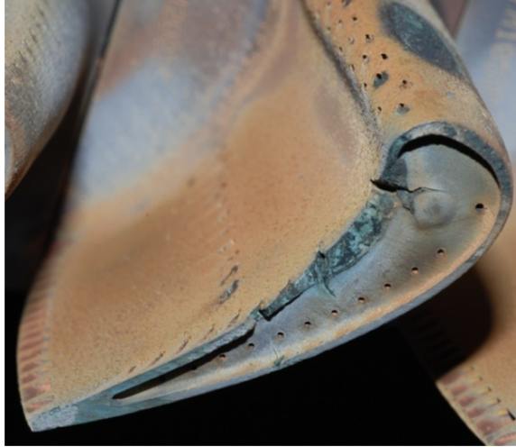
Figure 12: Turbine blade with excessive wear at the tip.
