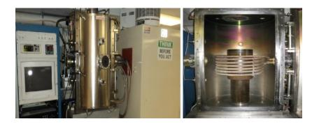
Figure 3.1 Hot Wall RF reactor outside (left) and inside (right) of growth reactor showing induction coils and graphite crucible.
