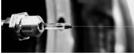
Figure 3.4: A liquid micro-jet in action producing a liquid water target in vacuum which allows photoelectrons to escape from the surface and reach an electron analyzer. Photo provided by the courtesy of Ev Henke.
