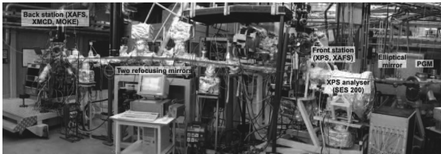
Figure 6.1. Beamline D1011 at MAX-lab in Lund. The red line indicates the path travelled by the x-rays [33].
