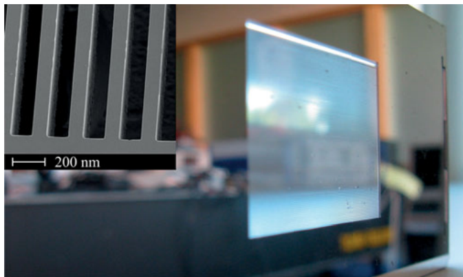
Figure 23. Photo of a beamsplitter as used in the Fourier transform spectrometer. The insert shows a scanning electron microscope picture of the reflective bars and slits, repeating with a period of about 200 \mu\text{m} .
