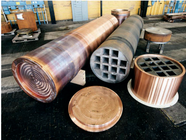
Figure 3.1: Image of sealed (left) and unsealed (right) copper canisters. In the unsealed canister the cast iron inset, which will be inside the copper layer, is visible. The spent nuclear fuel will be stored inside the squared openings in the cast iron. The image is from the Swedish Nuclear Fuel and Waste Management Company, SKB
