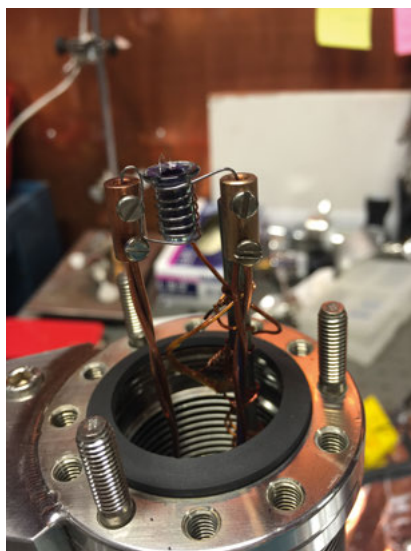
Figure 6.2. The evaporator used for CoPc deposition. Similar evaporator set-up was also applied to m-MTDATA and melamine depositions.
