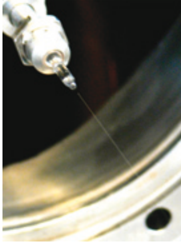
Figure 5.1: The liquid micro-jet with a diameter of approximately 15 micron.
