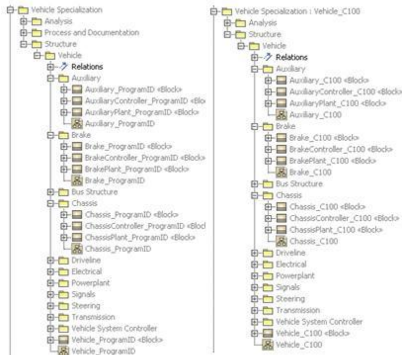
Figure A 1. (a) Vehicle Specialization package with generic “_ProgramID” block names. (b) C100 Specific Vehicle Package with specific “_C100” block names.
