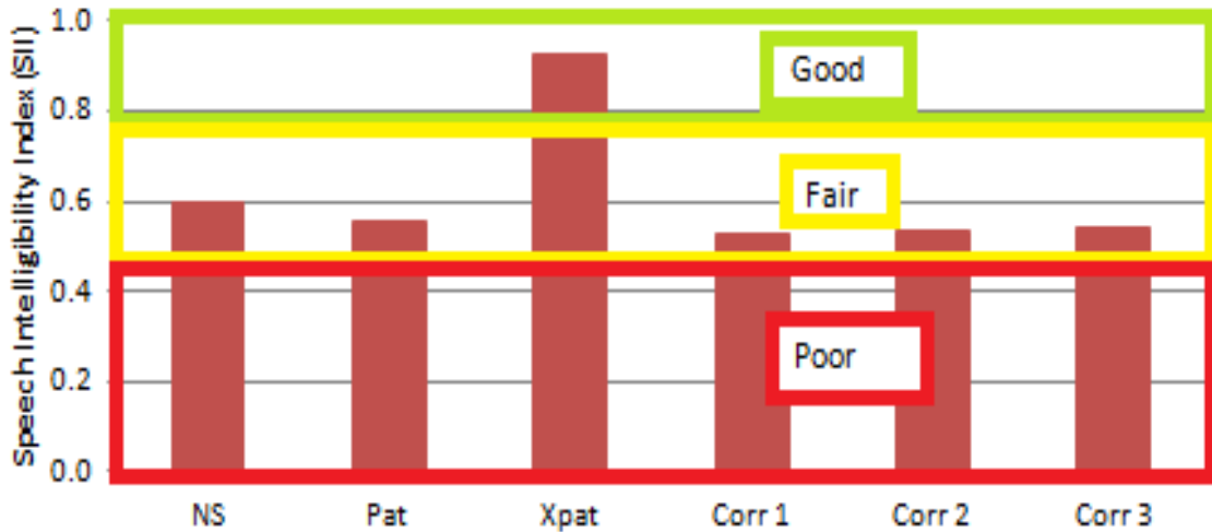
Appendix A. 10: Speech Intelligibility Index (SII) at various locations within hospital 3 Intensive Care Unit. Shown here are the ranges of SII: “poor” (0-0.45), “fair” (0.45-0.75) and “good” (0.75-1.0).
