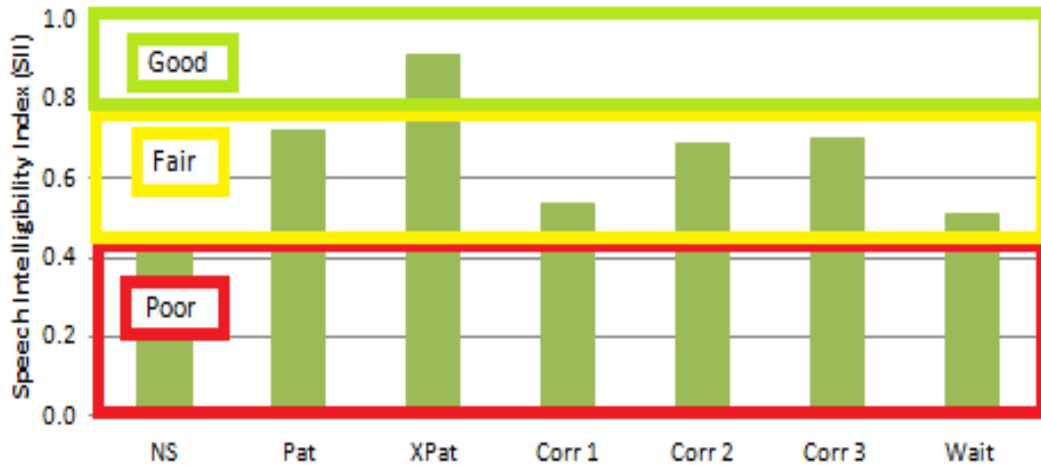
Figure 45: SII shown by location in hospital 2 MB unit. Shown here are the ranges of SII: “poor” (0-0.45), “fair” (0.45-0.75) and “good” (0.75-1.0).
