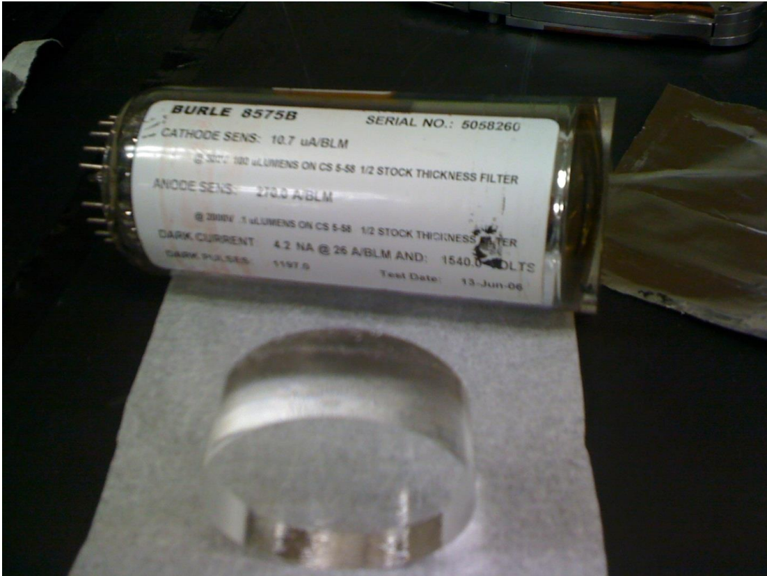
Figure 11. BURLE 8575B photomultiplier tube and the light pipe shown are installed between the NE-213 detector and the ORTEC 265A Photomultiplier Base Assembly.
