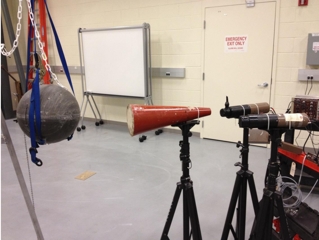
Figure 9. Paraffin shadow shields with steel bases are used to attenuate all radiation from the measurement and arrive at the background due to room-returned and air scattered neutrons.
