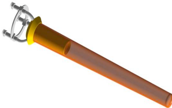
Figure 2.9: Schematic diagram of the 40-cm long \text{LD}_2 target cell used in the g13 experiment. The figure is from [53].
