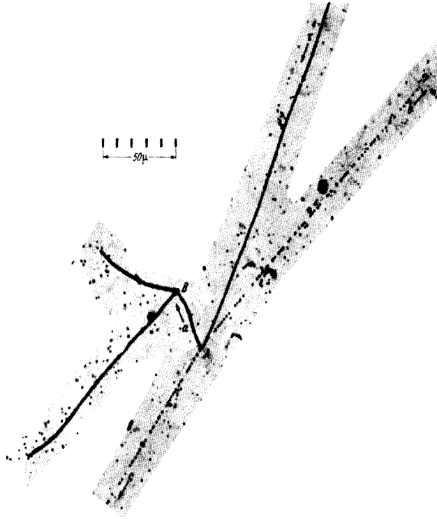
Figure 1.3: Discovery of K^+ . K^+ decays to double \pi^+ and \pi^- . The figure is from [1].
