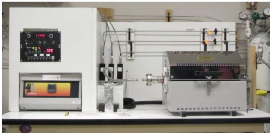
Figure 2.1 The home-built CVD graphene synthesis system
