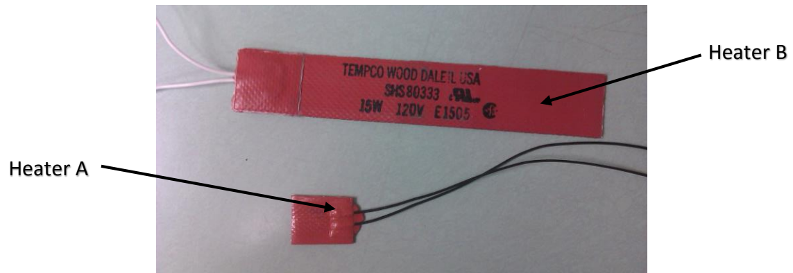
Figure 3.7 Heaters A and B
