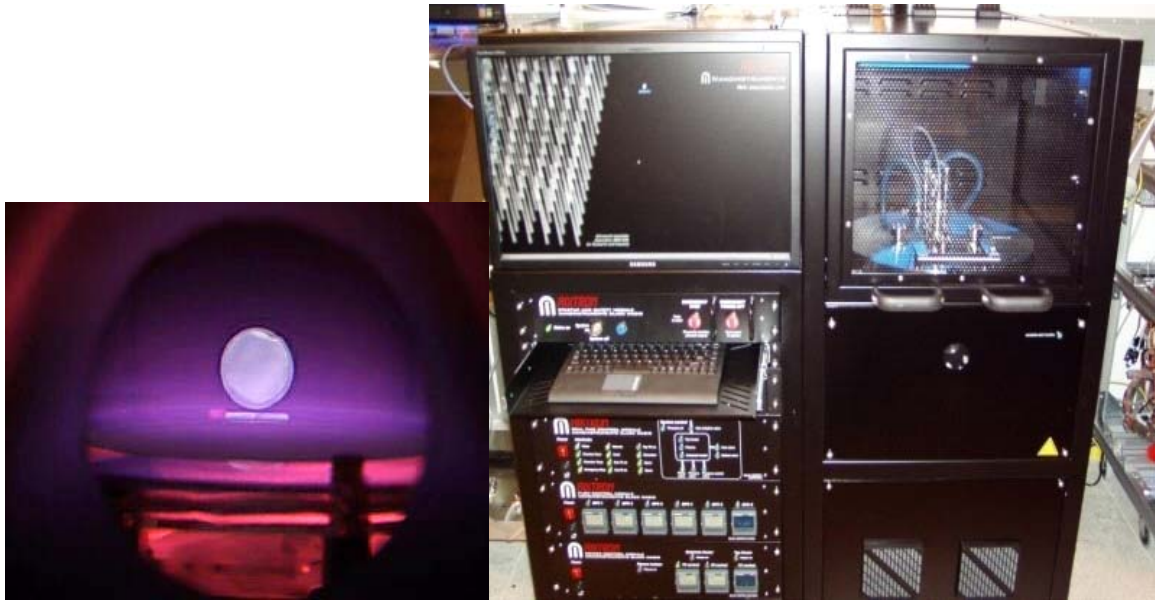
Fig. 3.1. Black Magic Pro 4'' CVD system. Left: growth chamber when plasma in on, and right: the outside look of the system.
