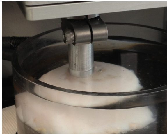
(e) Stress-relaxation analysis of cartilage plug with tribometer
