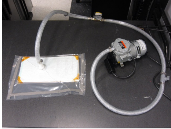
Figure 16. Vacuum bonding process setup showing the vacuum pump and the curing setup in a sealed plastic bag.
