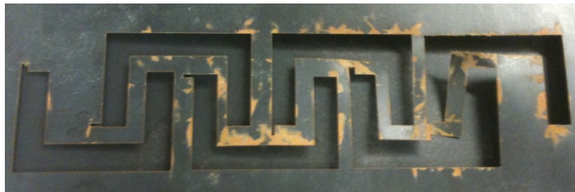
Figure 5.6 Oxidation occurring on electric steel after abrasive waterjetting, despite prompt removal of water via compressed air.
