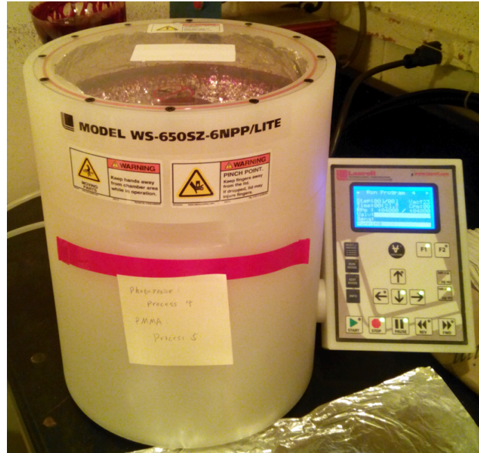
Figure 4.2: Spin coater machine.
