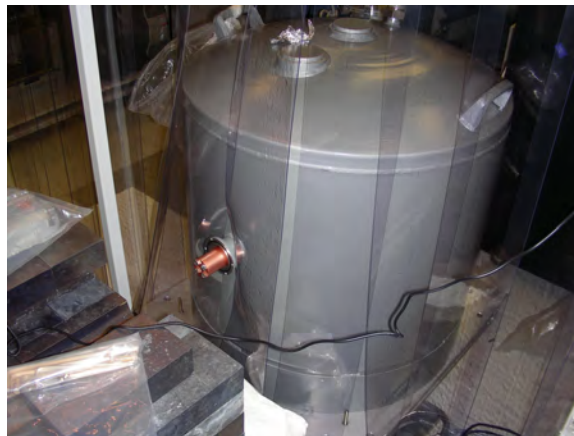
FIGURE 3.8. The liquid nitrogen dewar of Cascades prior to being attached to the lower cryostat with a thermal connection
