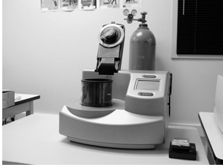
Figure 4.1. RF/DC 13.56 MHz frequency sputtering unit used for metallization.
