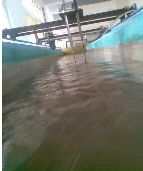
Figure 3.6. Photo of movable bridge used for Experimentation.
