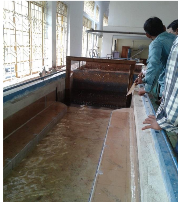
Figure 3.4. Photo of Inlet mouth section
