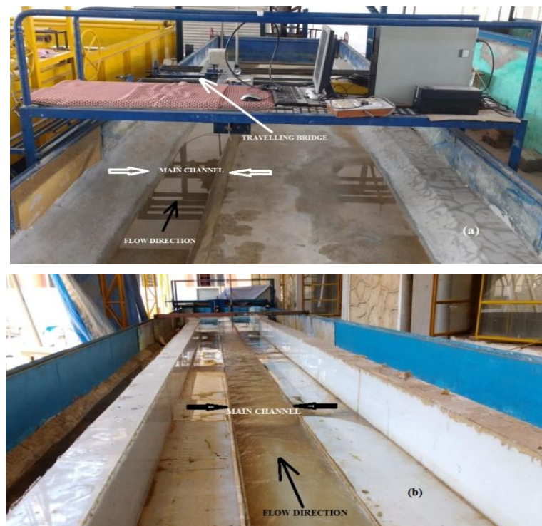
Figure 3.1: Photo of fabricated experimental channels (a) Trapezoidal (b) Rectangular
