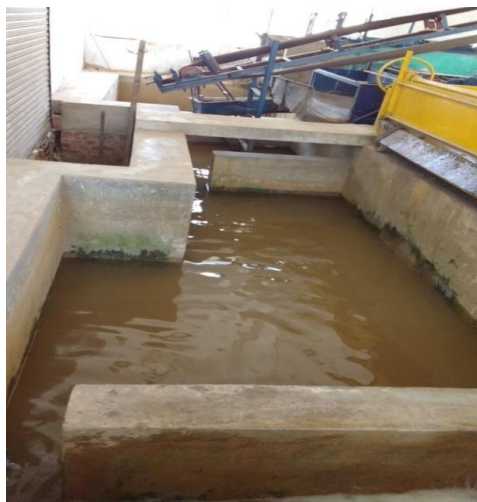
Figure 3.6: Photo of Volumetric tank and vertical piezometer
