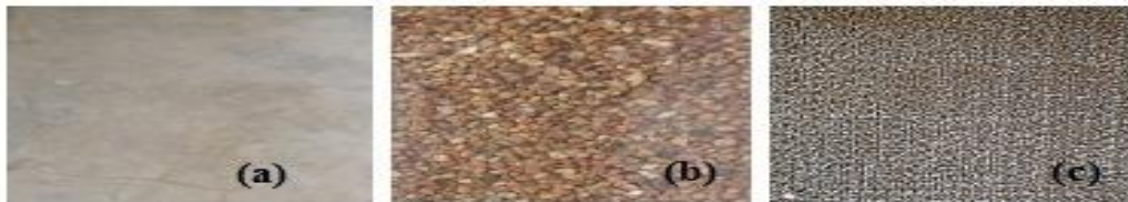
Figure 3.12: Different roughness materials used in trapezoidal channel (a) cement concrete trowel finished (b) Small Gravel (size 7 to 20 mm) (c) Plastic mat (15mm thick)
