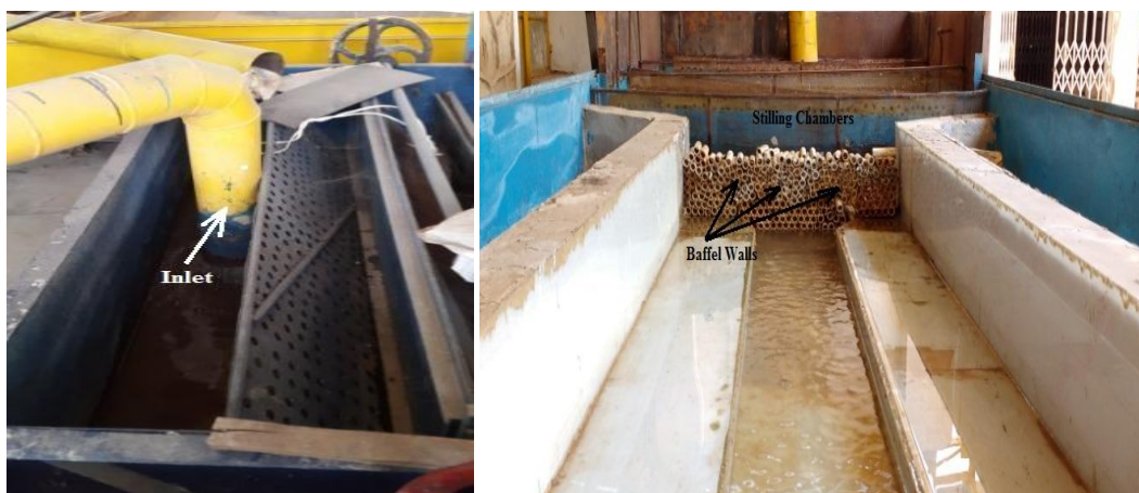
Figure 3.4: Photo of Experimental channel with arrangement of stilling chambers and baffle walls
