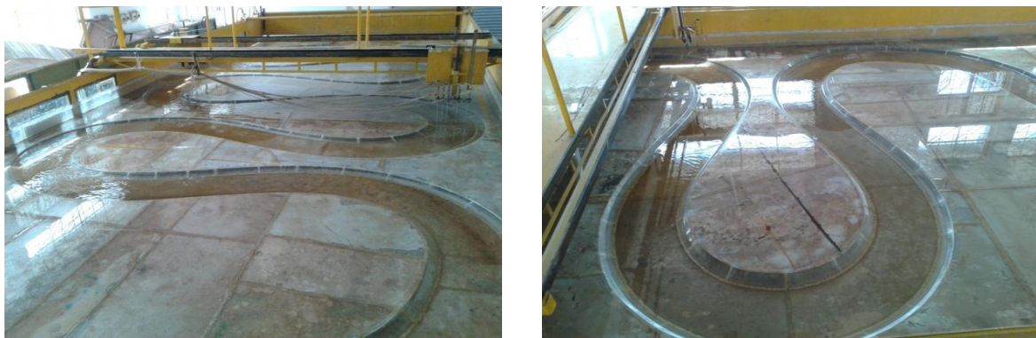
Fig. 3.6 meandering channel inside the flume with measuring equipment
