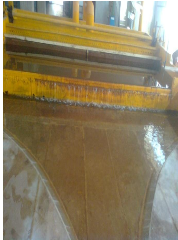
Photo.3.1 (a) View of Experimental Channel Photo.3.1 (b) Rectangular Notch
