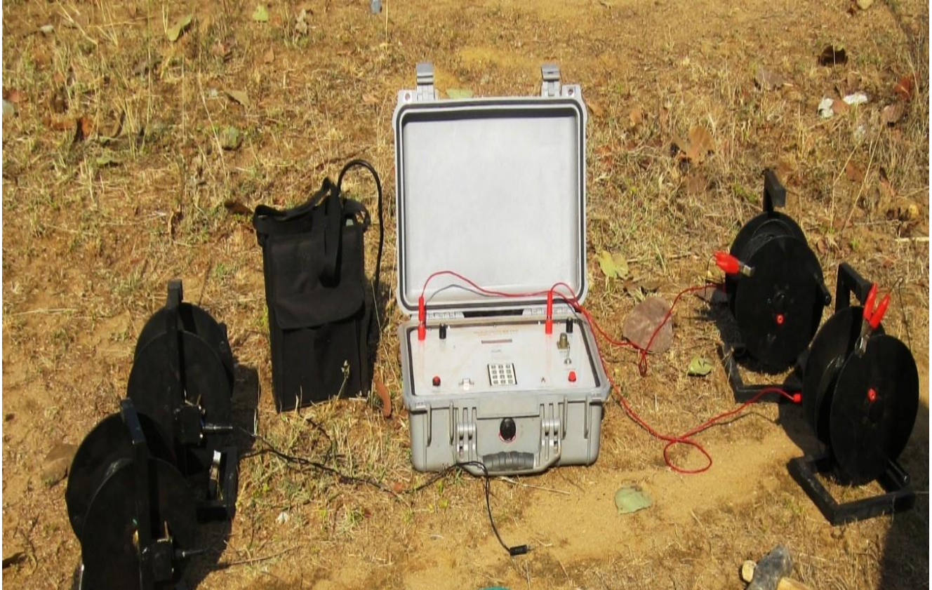
Figure: Vertical electrical sounding, Department of mining engineering, NIT Rourkela
