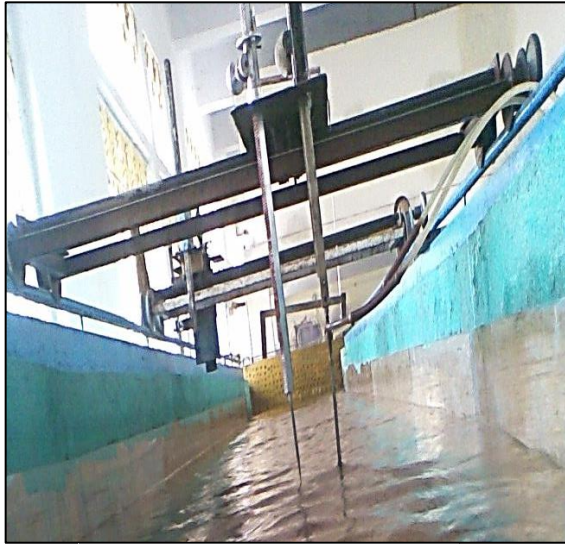
(iii) Point gauge and Pitot tube measuring velocity
