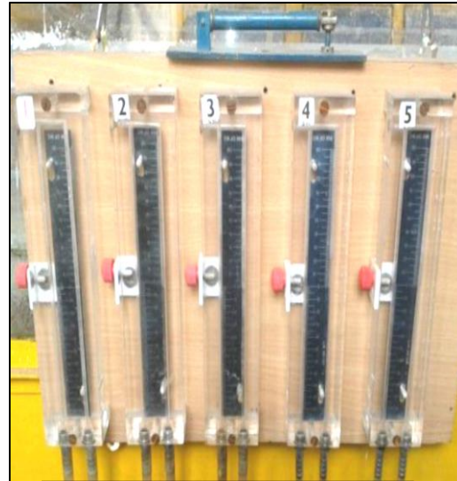
(iv) Series of manometer used for measuring pressure
