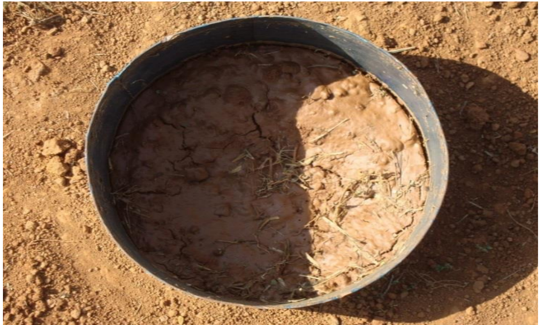
Fig.4.1.1: Single Ring Infiltrometer of 30cm diameter
