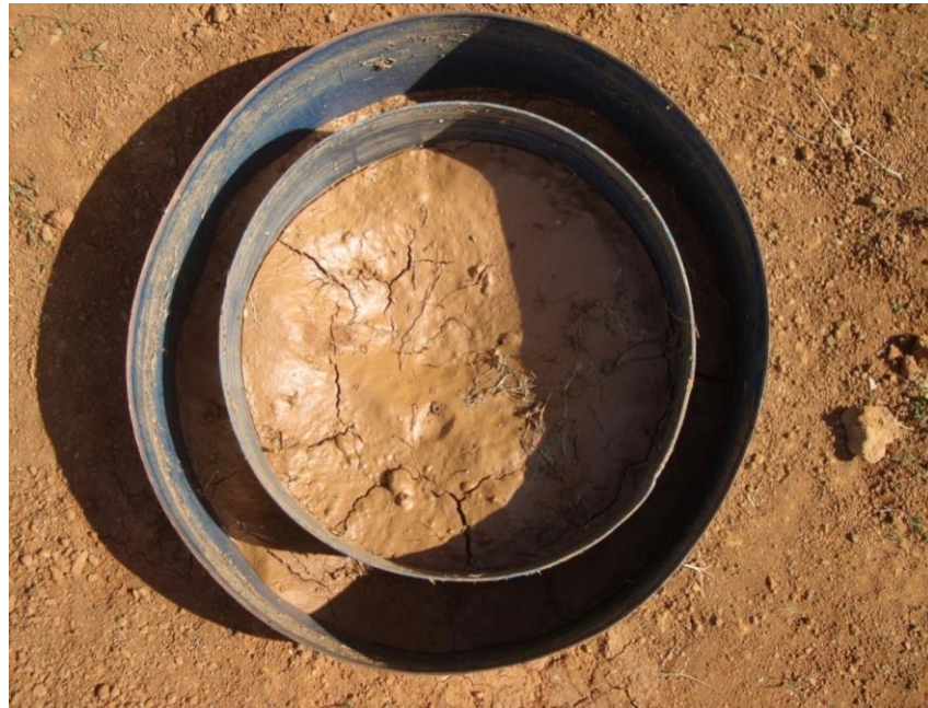
Fig.4.2: Double-Ring Infiltrimeter of 45-60cm diameter rings
