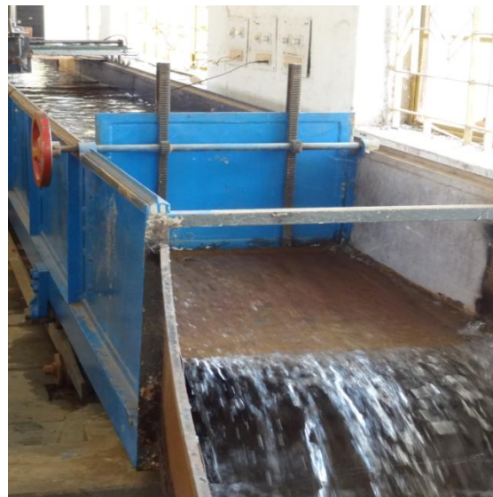
Fig 3.9 photo of channel outlet
