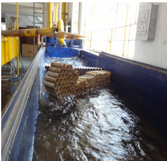
Fig 3.8 photo of channel inlet along with Straightners
