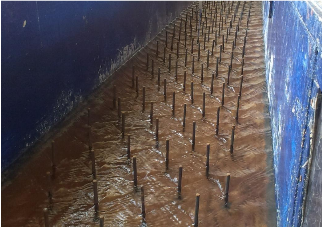
Fig 3.4 channel with unsubmerged flow
