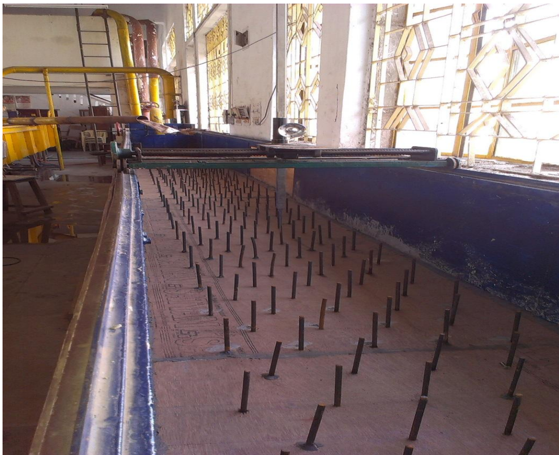
Fig 3.3 photo of vegetated open channel
