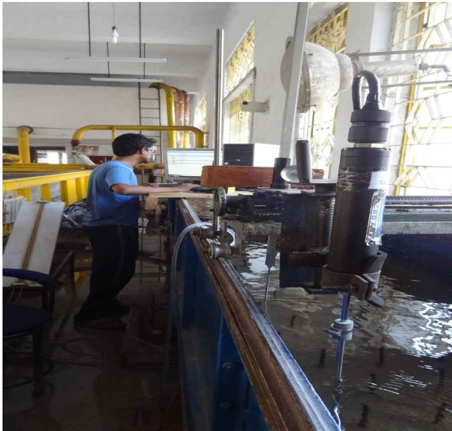
Fig 3.10 ADV setup in the channel
