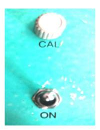
"CAL" knob: The calibration of the instrument is done with this knob.once the instrument is calibrated for a particular range this knob should not be disturbed. Till the required set of the reading is obtained for that range
