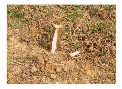
The finalised spot is considered as a centre for the 4 pin readings.
