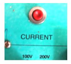
**Voltage selector**: This switch is located below the current push button .the output AC voltage (50 /100/200/400 VAC) is to be selected with this selector switch, at different stages.
