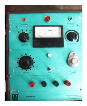
**Current indicator**: At the left hand corner is the Red push button marked as "CURRENT". While operating the instrument when this button is pressed the meter indicates the current that is being penetrated in the ground (between P1 and P4 circuit).if the meter indicates say 20 that means the actual current flowing is 50 milliamps (2.5 times of the meter reading)
