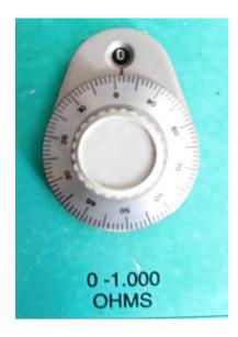
In short the reading obtained on the ten turn pot is to be multiplied with the selected range ,to get the actual reading.
