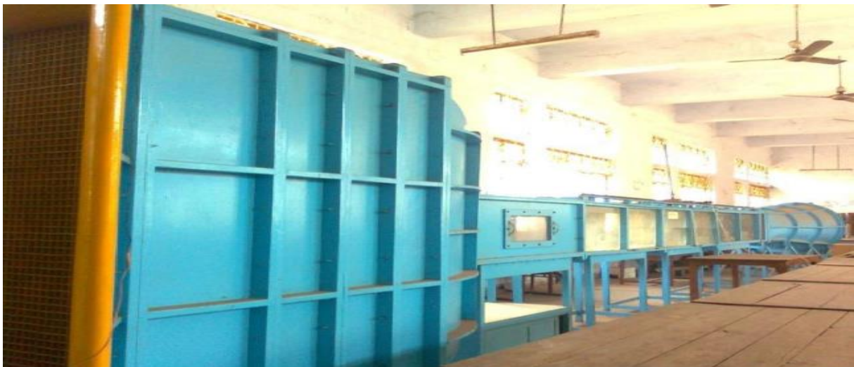
Fig.3.1: Low Speed Wind Tunnel
