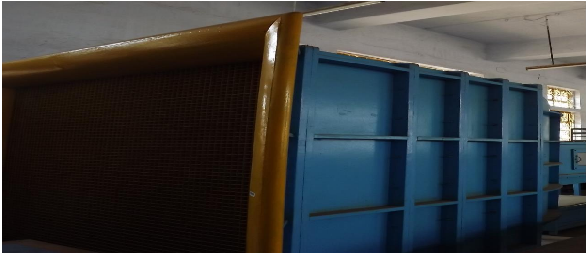
Fig.3.2: Effuser zone of the Low Speed Wind Tunnel
