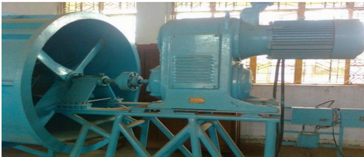
Fig.3.4: Driving Unit of the Low Speed Wind Tunnel
