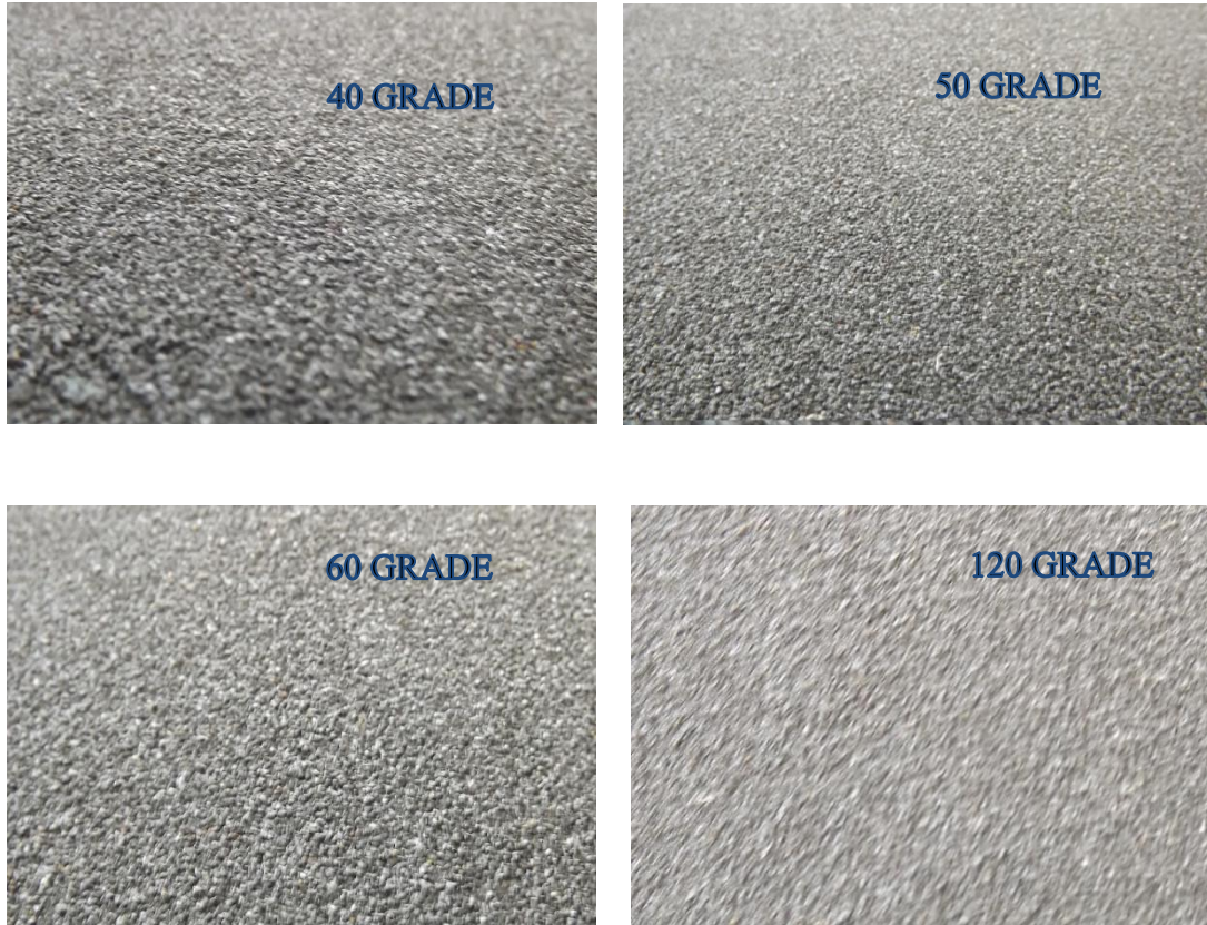
Fig: 3.7: flat plate with roughness 40 grade( 375\mu\text{m} ), 50 grade( 345\mu\text{m} ), 60 grade( 290\mu\text{m} ), 120 grade( 125\mu\text{m} ) respectively
