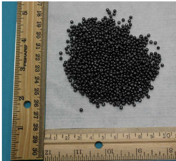
Figure 2.9. Sample#1 Se-As master alloy wet shots As-9.5%.
