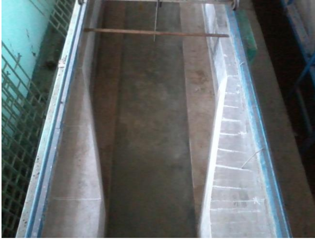
Fig.3.5 Non prismatic section of the channel
