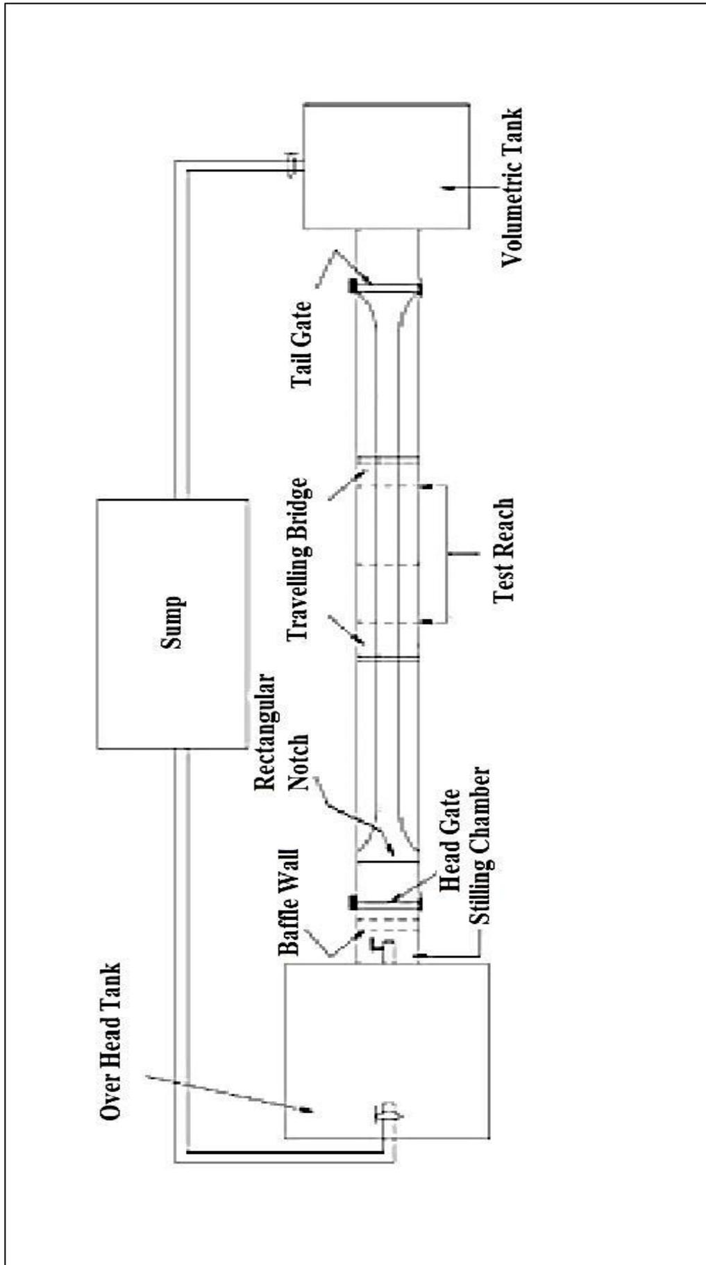
Fig. 3.1 Plan view of the experimental channel
