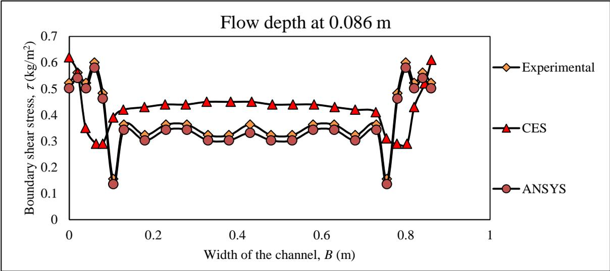
Fig. 5.3.c. Comparison of Boundary shear stress distribution for flow depth 0.086m
