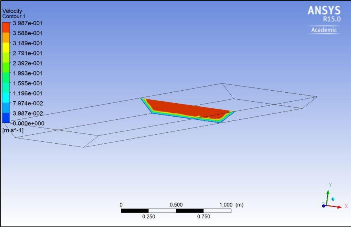
Fig. 5.2.c longitudinal velocity contour of flow depth 0.086 m using ANSYS
