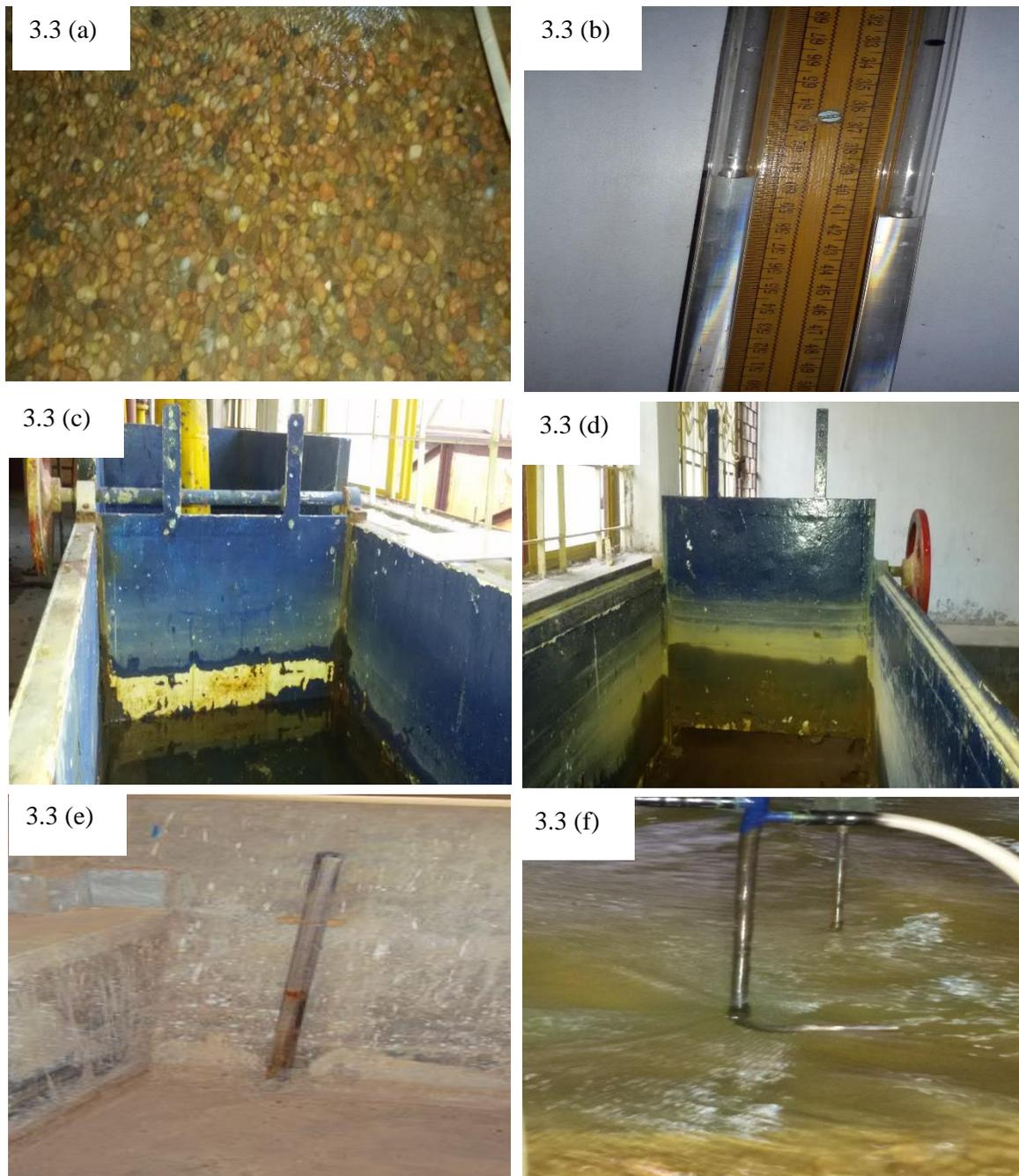
Fig. 3.3 Photographs of experimental procedure (a) Gravel bed (b) Manometer fitted with scale (c) Head gate (d) Tail gate (e) Piezometer (f) Pitot tube and Point gauge fitted in travelling bridge arrangements
