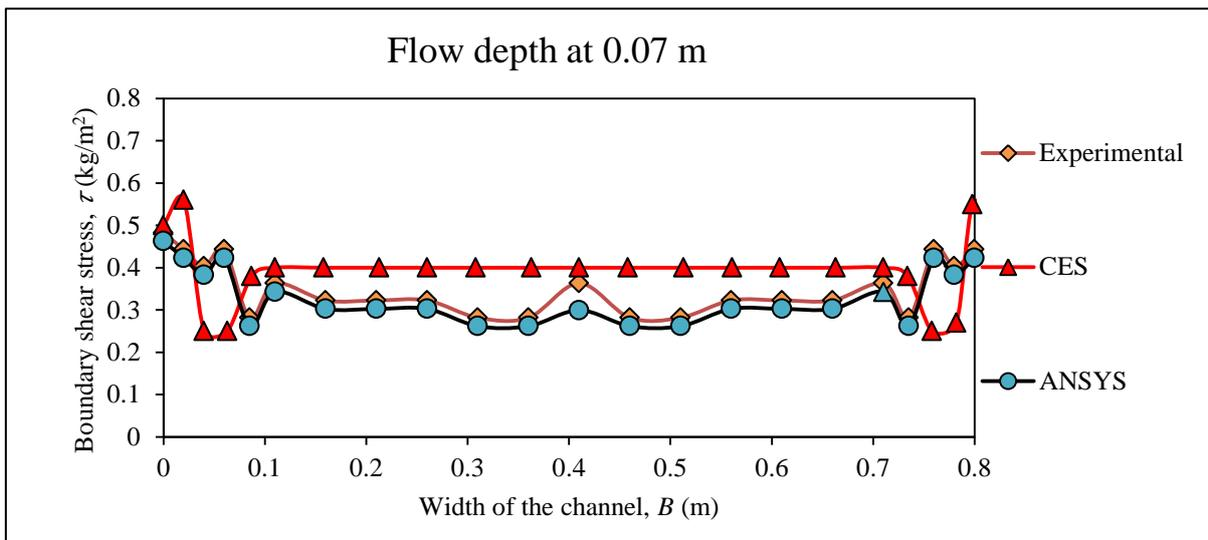
Fig. 5.3.a. Comparison of Boundary shear stress distribution for flow depth 0.07m
