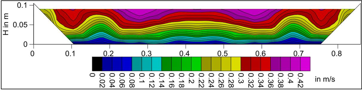
Fig. 5.1.d. longitudinal velocity contour of flow depth 0.0916 m
