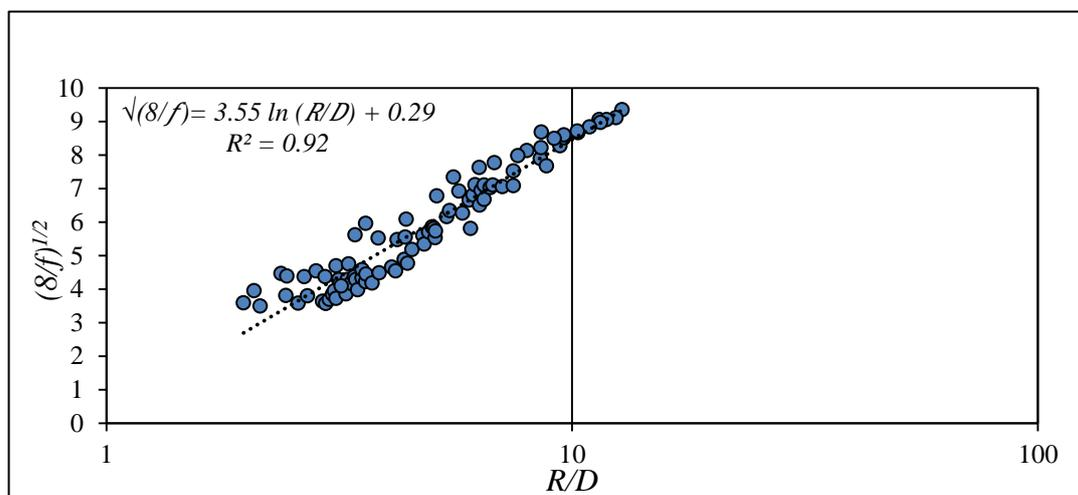
Fig.5.9. Friction factor variation for intense load condition
