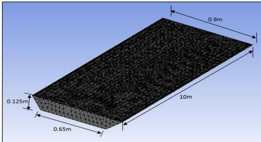
Fig. 4.4 Experimental channel Meshed create using ANSYS
