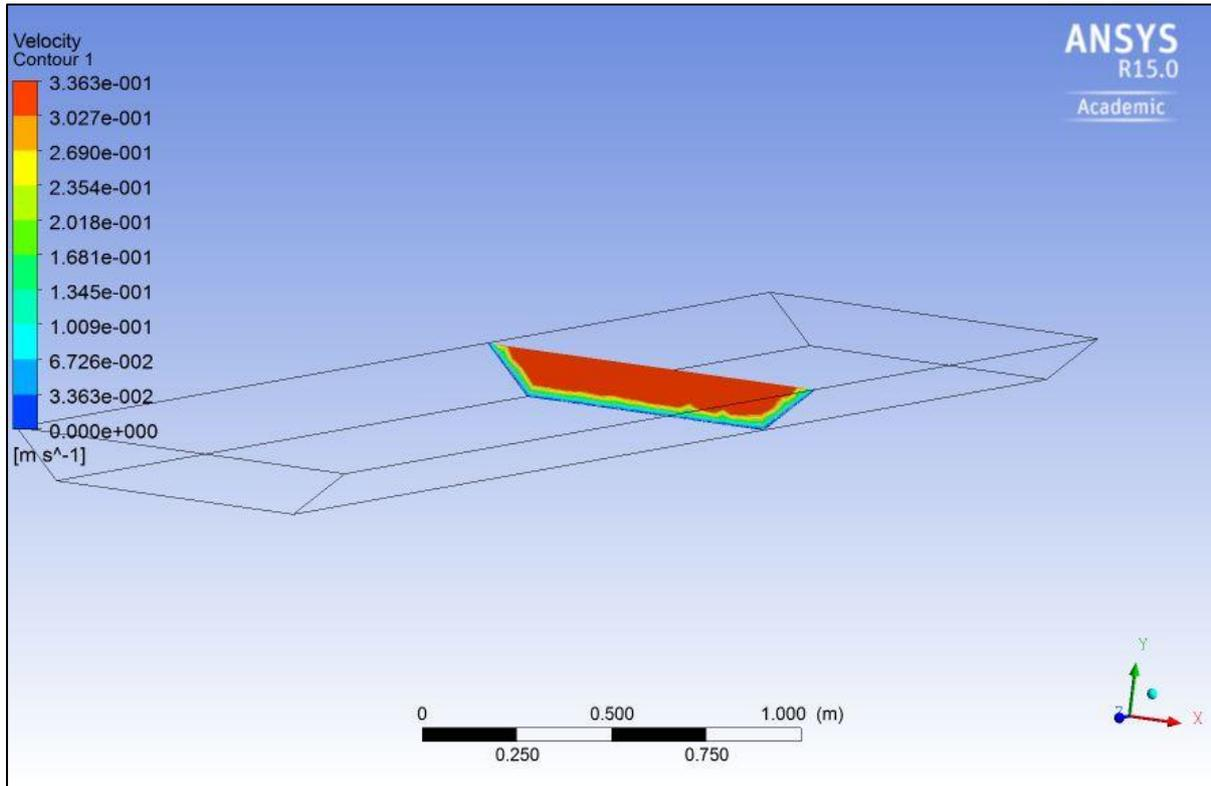
Fig. 5.2.a longitudinal velocity contour of flow depth 0.07 m using ANSYS
