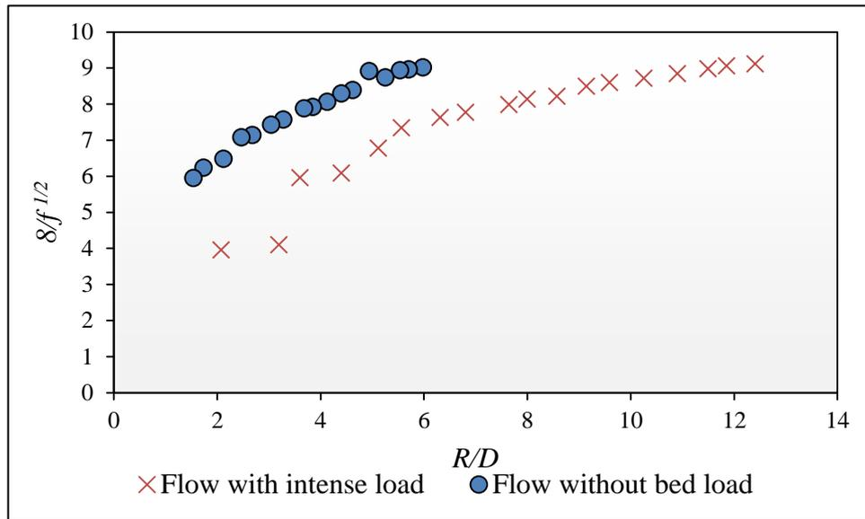
Fig. 4.1 Variance of friction factor for both bed load conditions
