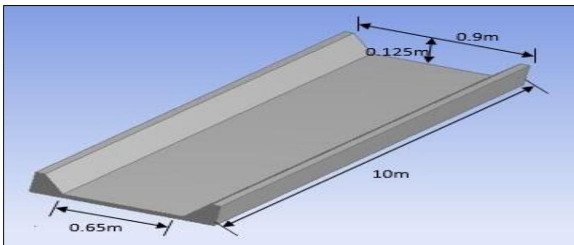
Fig. 3.2 Overall view of the flume with experimental set up
