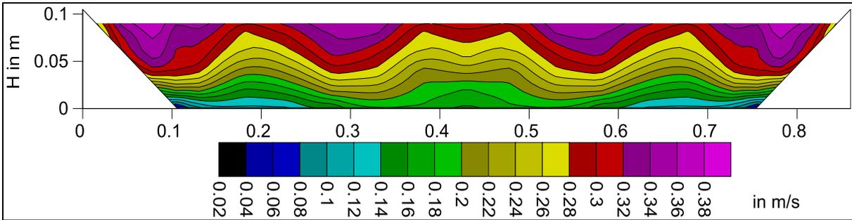
Fig. 5.1 b. longitudinal velocity contour of flow depth 0.08 m
