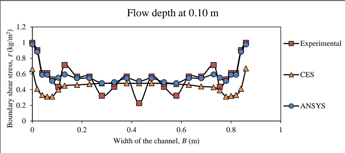
Fig. 5.3.e. Comparison of Boundary shear stress distribution for flow depth 0.10 m
