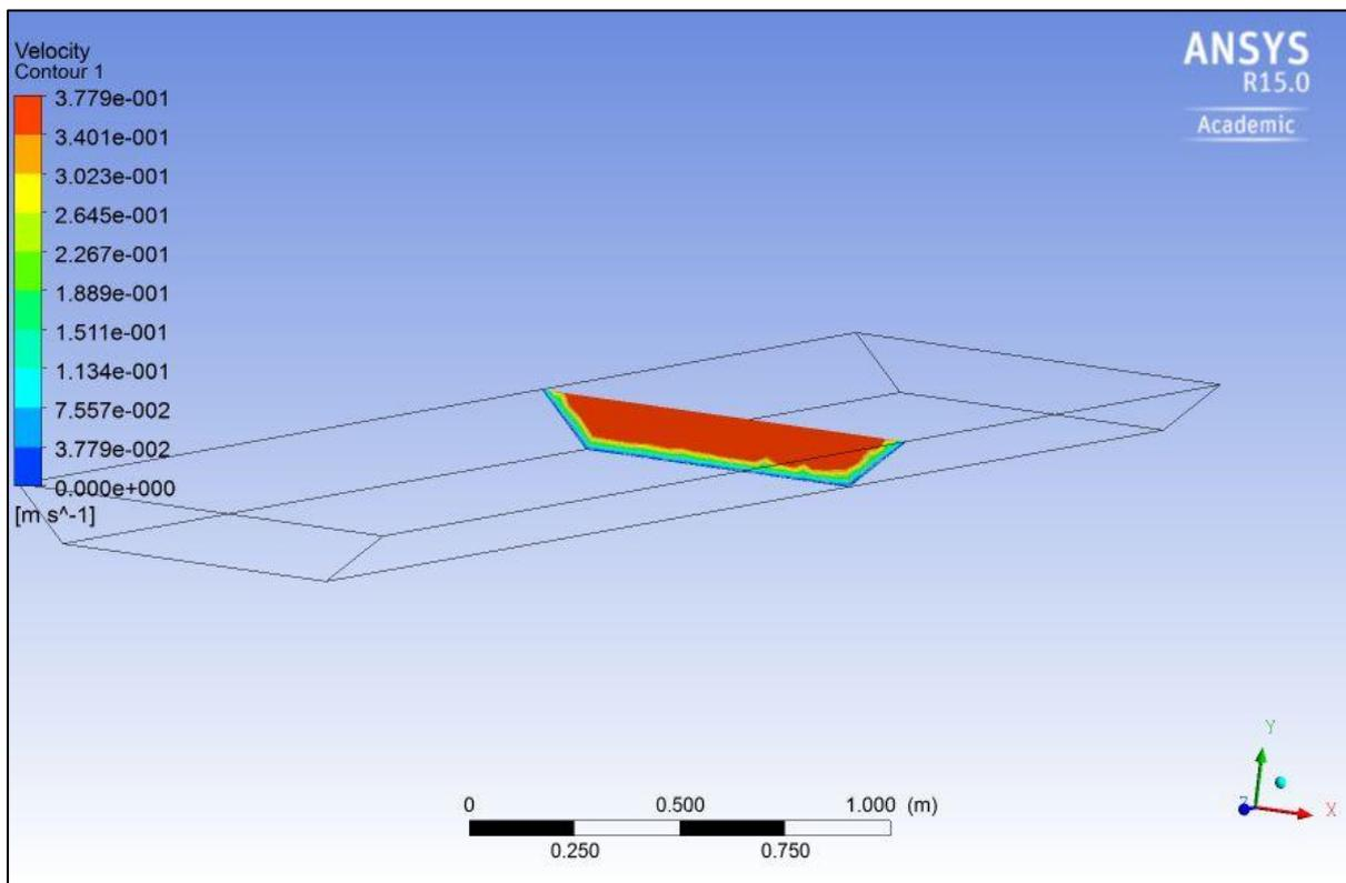
Fig. 5.2.b longitudinal velocity contour of flow depth 0.08 m using ANSYS
