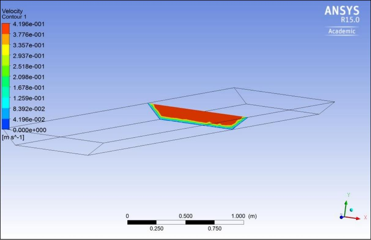
Fig. 5.2.d longitudinal velocity contour of flow depth 0.0916 m using ANSYS
