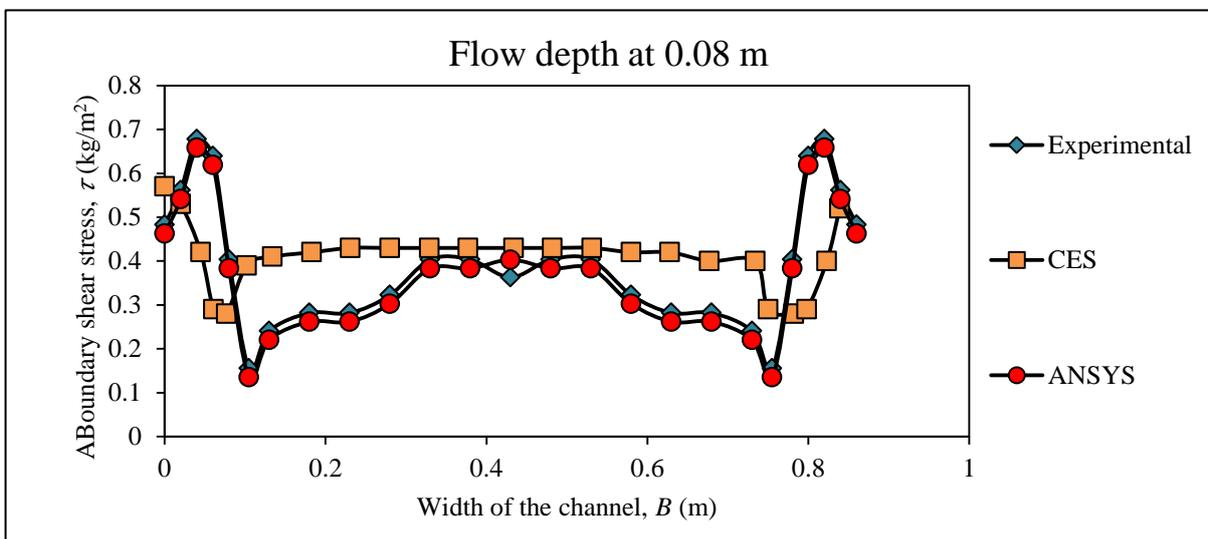
47 | Page Fig. 5.3.b. Comparison of Boundary shear stress distribution for flow depth 0.08m
