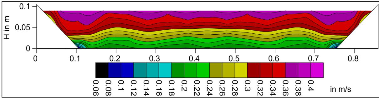
Fig. 5.1 c. longitudinal velocity contour of flow depth 0.086 m
