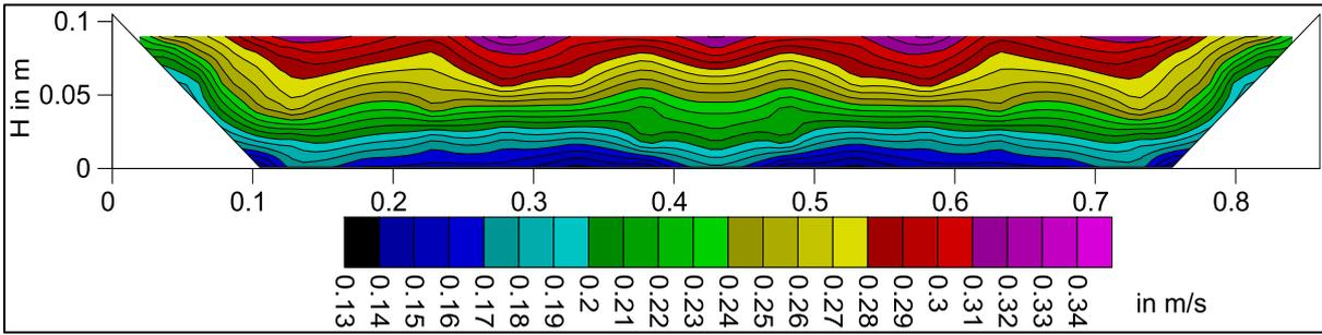
Fig. 5.1 a. longitudinal velocity contour of flow depth 0.07 m
