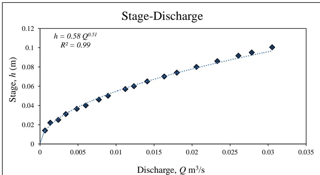
Fig.5.8. Stage-discharge relationship for intense load condition
