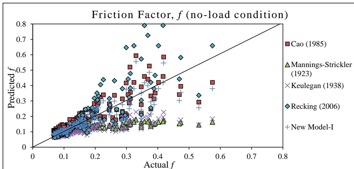
Fig.5.6. Validation of friction factor model for no load condition with other author data
