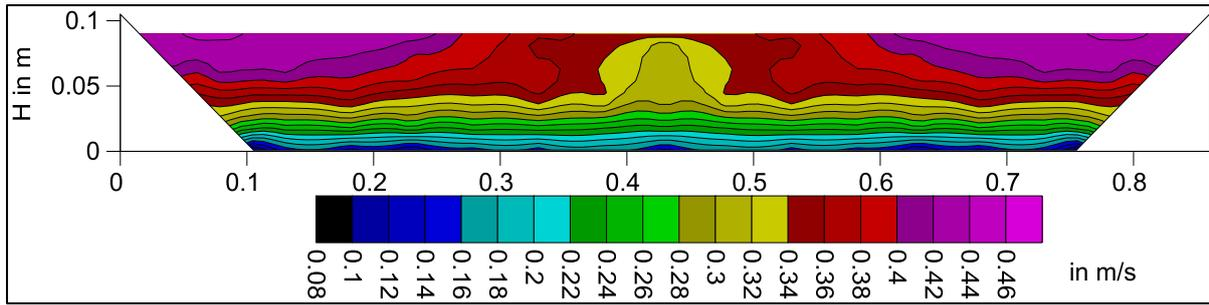
Fig. 5.1.e. longitudinal velocity contour of flow depth 0.10 m
