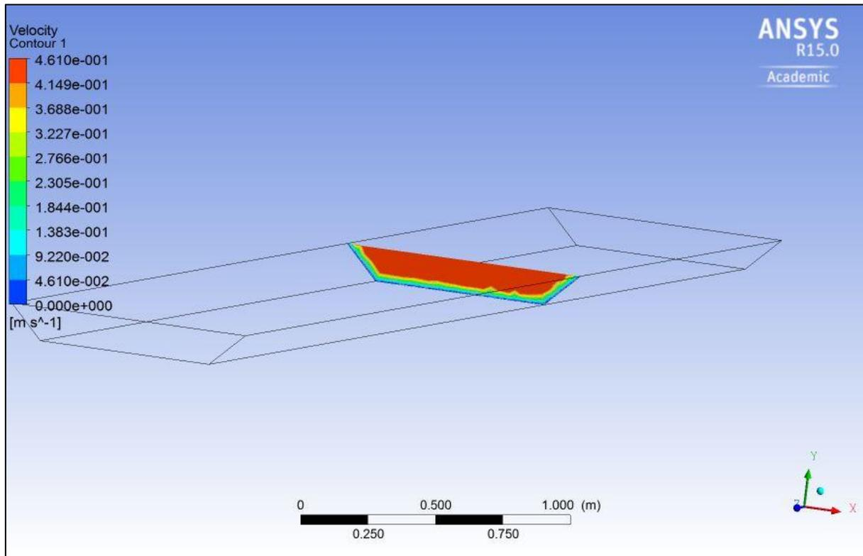
Fig. 5.2.e longitudinal velocity contour of flow depth 0.10 m using ANSYS
