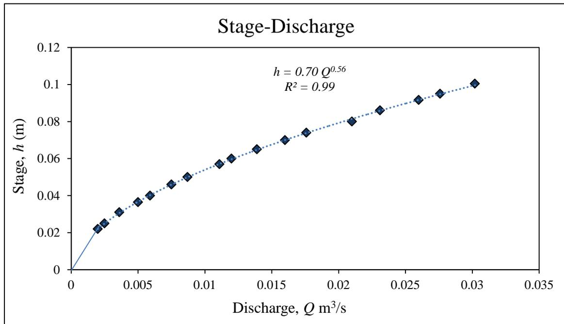
Fig. 5.4. Stage-discharge relationship for no load condition
