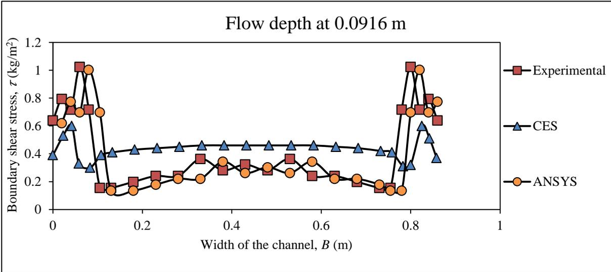
Fig. 5.3.d. Comparison of Boundary shear stress distribution for flow depth 0.096m
