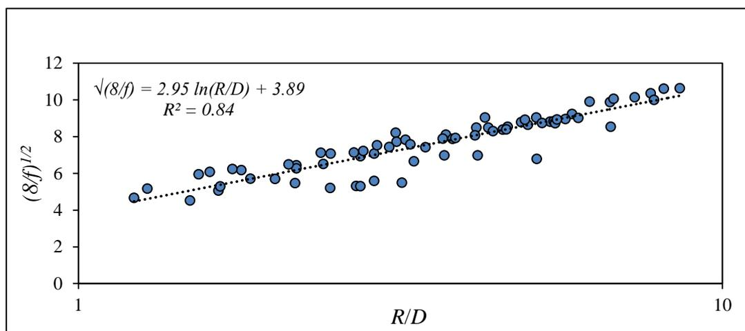
Fig. 5.5. Friction factor variation for no load condition
