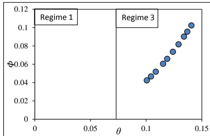
Fig. 4.2 Measured bed load intensity in relation to dimensionless shear stress
