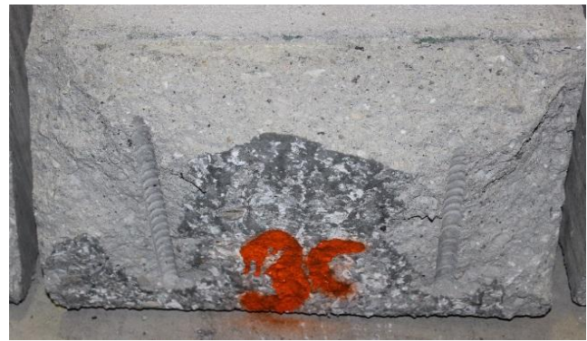
d) Bond interface (overlay concrete)
