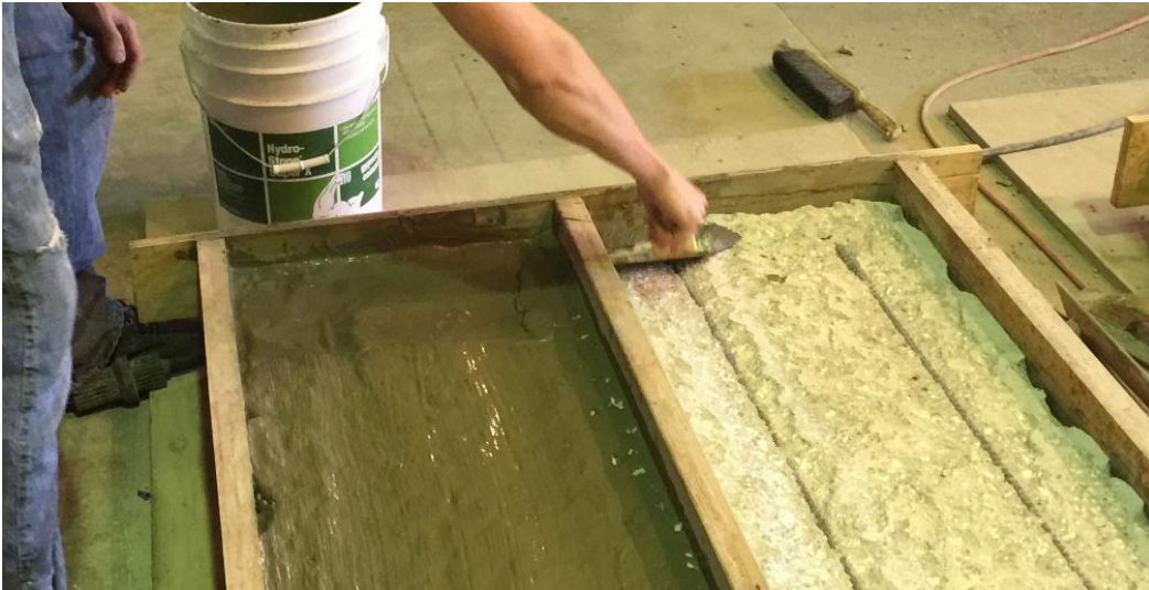
Figure 84. Application of grout to positive bending flexural test specimen (Case 1)
