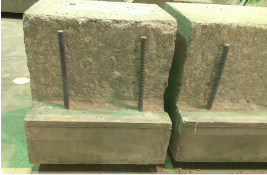
Figure 67. Pair of push-out test sub-specimens after concrete removal (Case 4)
