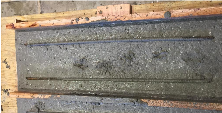
Figure 82. Positive bending flexural test specimen after substrate concrete placement (Case 4)
