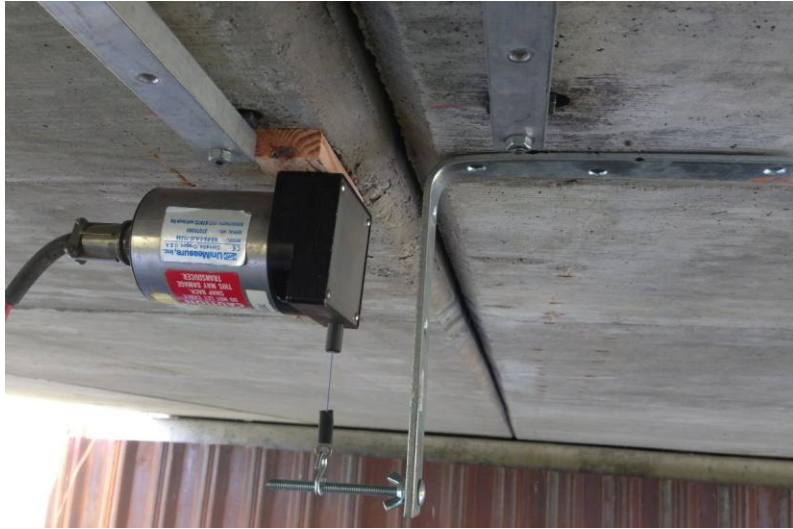
Figure 29. Relative displacement gage setup
