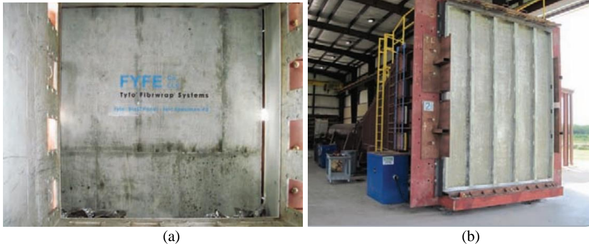
Figure 2.7 Blast Panels of Fyfe Co. in its tested specimen (a) interior, and (b) exterior [52]
