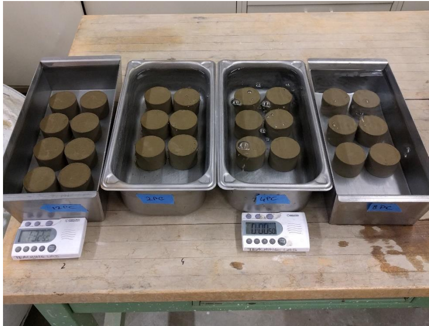
Figure E1. Wetting period of W-D test
