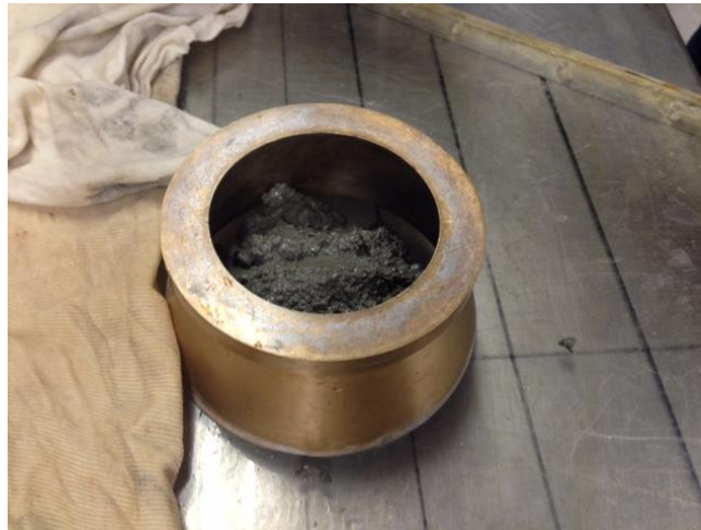
Figure 10. Mold and smooth plate for flowability test
