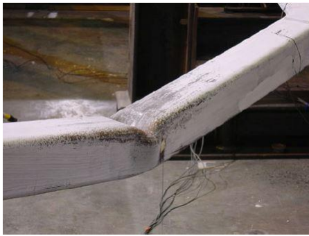
(c) Local buckling of the tested brace
