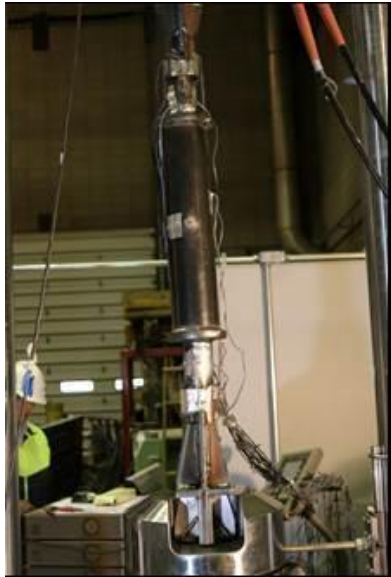
(c) Out-of-plane buckling shape
