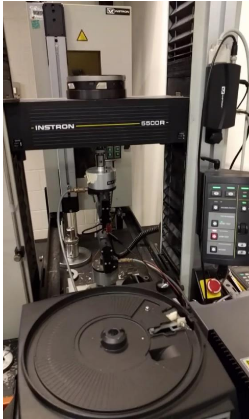
Figure 4.11 Tension setup for perovskite solar cell samples
