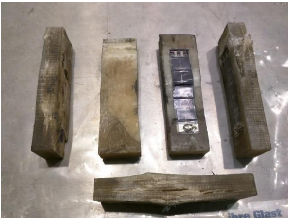
Figure 4.22 A-Si compression samples failure modes
