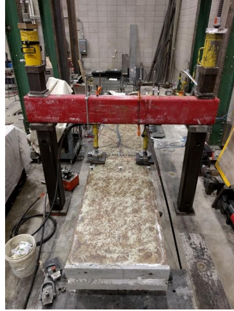
Figure 3.13 PVICS panel under three-point loading
