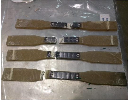
Figure 4.24 Failure modes for a-Si tension samples subjected to tension monotonic loading
