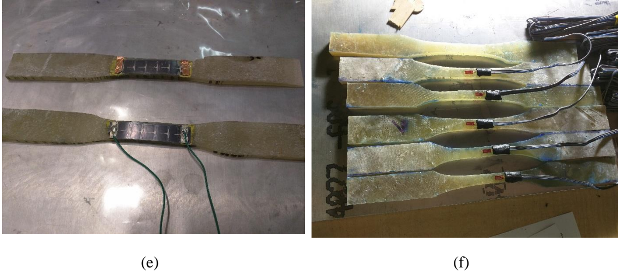
Figure 4.1 Sample preparation process (a) solar modules attached to peel ply, (b) sealed bag during curing process, (c) solar module attached to FRP plate, (d) Cutting compression samples, (e) Soldering wires to tension samples, (f) installing strain gages
