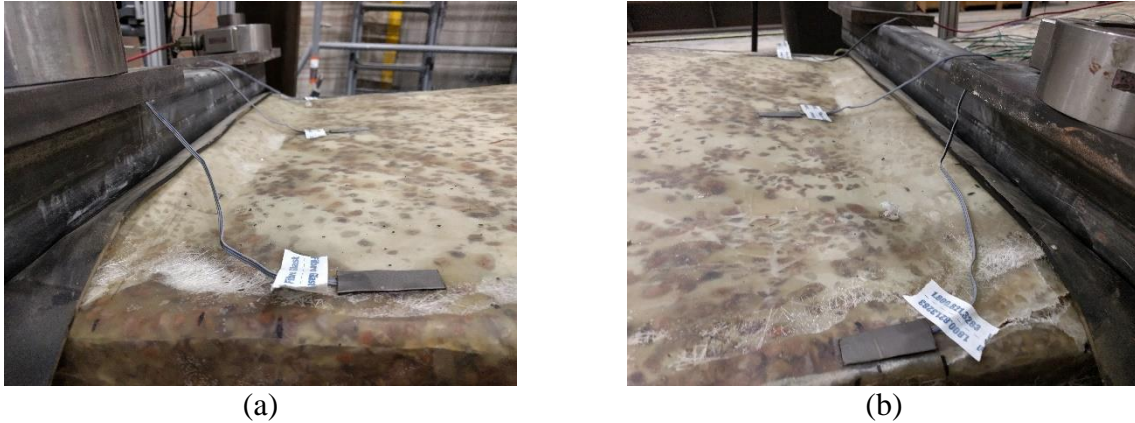
Figure 3.28 Wrinkling of the top FRP, (a) view for east side and from the (b) west side
