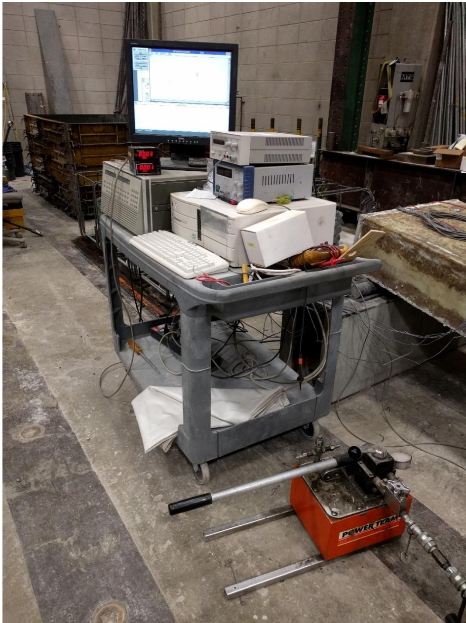
Figure 3.16 Strain, deflection and load data acquisition setup along with manual hydraulic jack
