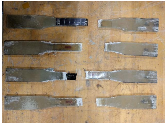
Figure 4.23 Failure modes for a-Si tension samples subjected to tension loading and unloading
