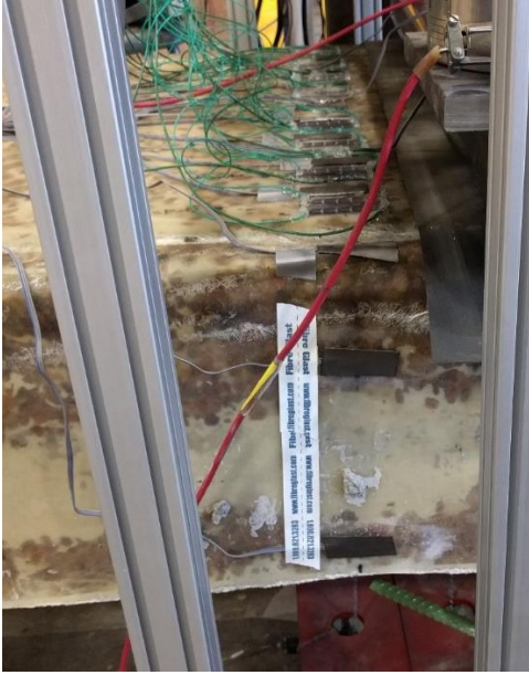
Figure 3.12 Side strain gages location
