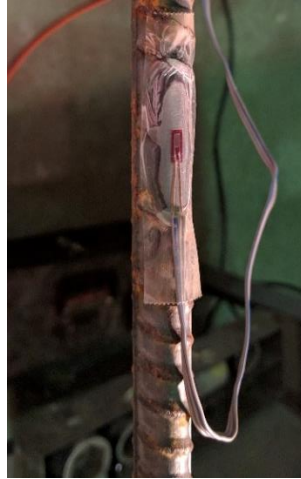
Figure 3.8 Installing strain gages
