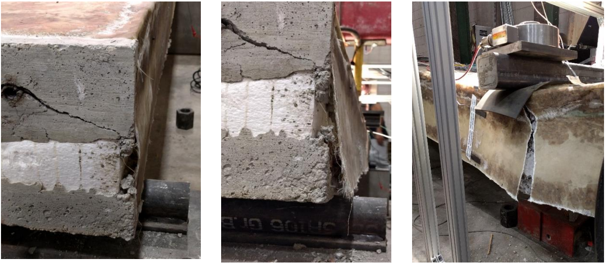
Figure 3.25 FRP shear connector failure; (a) Southwest side buckling, (b) debonding of shear connector at the southwest side, (c) Failure of shear connector at mid-span
