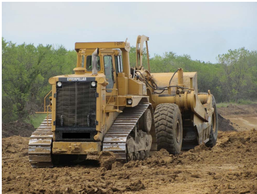
Figure 39. Warren County Project 2: Caterpillar MT-35 scraper used to collect and place loose fill materials
