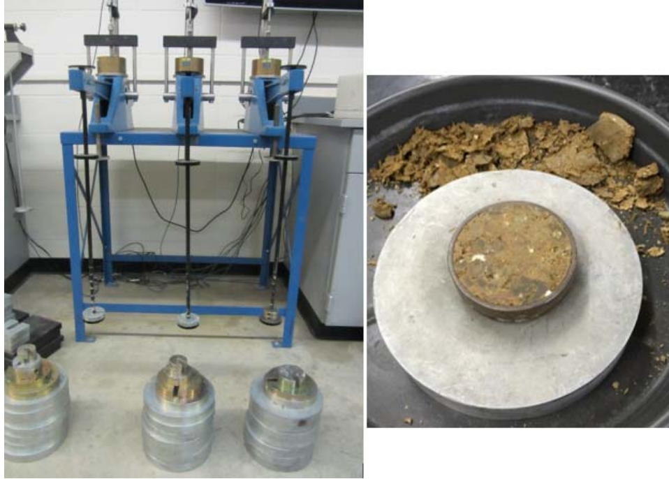
Figure 19. One-dimensional consolidation testing equipment and specimen
