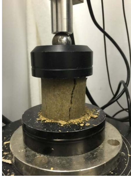
Figure 17. Specimen failure after measurement of UCS
