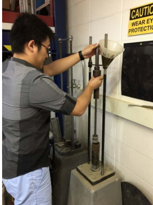
Figure 16. ISU 2 in. by 2 in. specimen compaction
