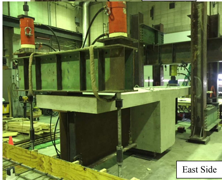
Figure 3-39. West and East Side Loading Configuration
