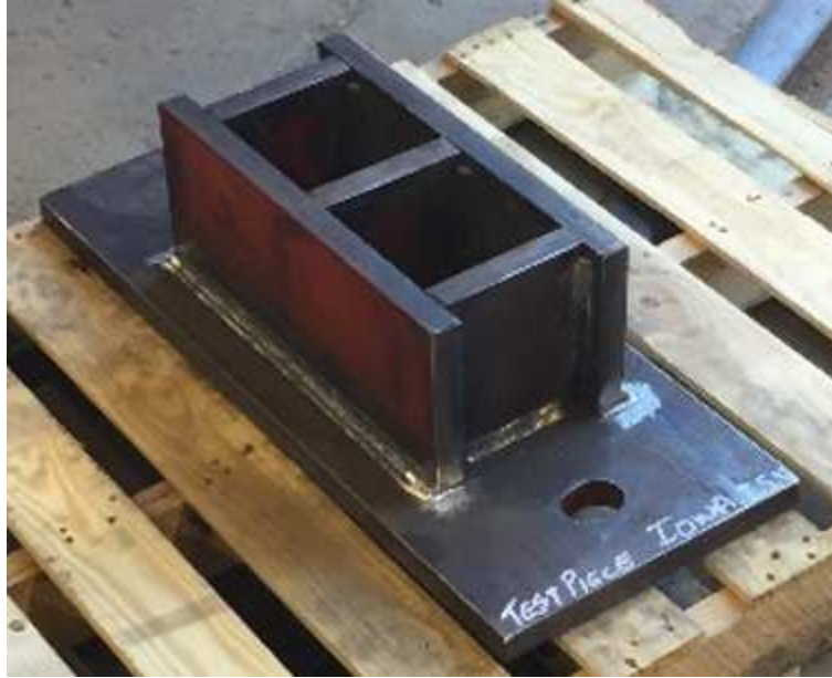
Figure 3-23. Fabricated Compression Block
