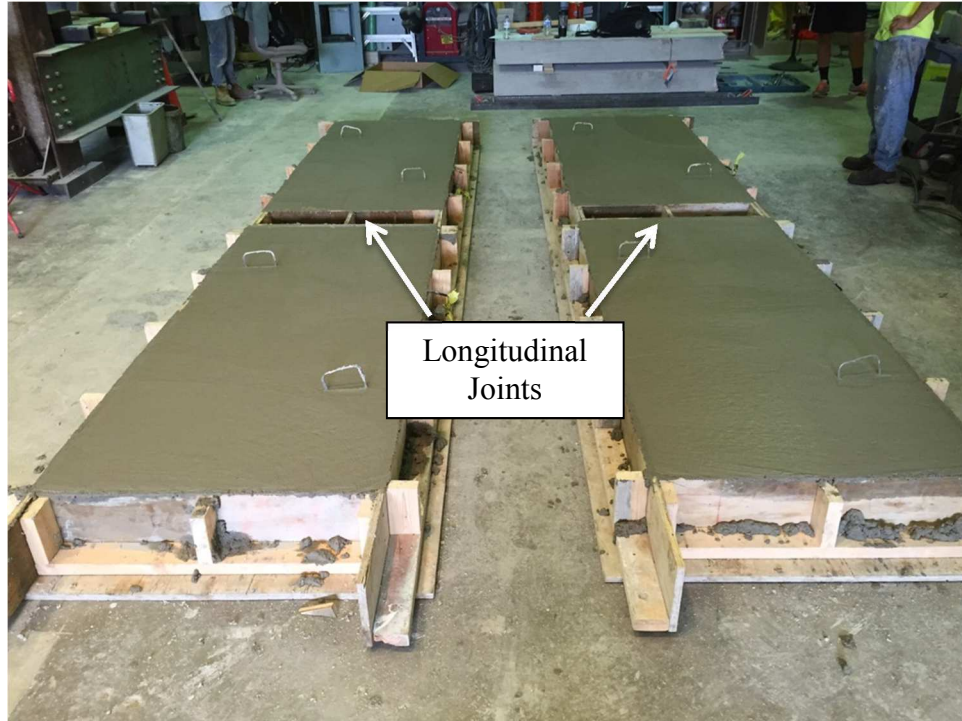
Figure 3-13. Placement of HPC for the Deck Panels
