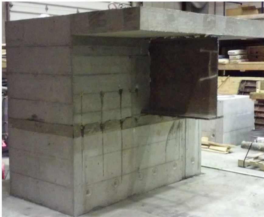
Figure 35. Completed grout bed and coupler grouting
