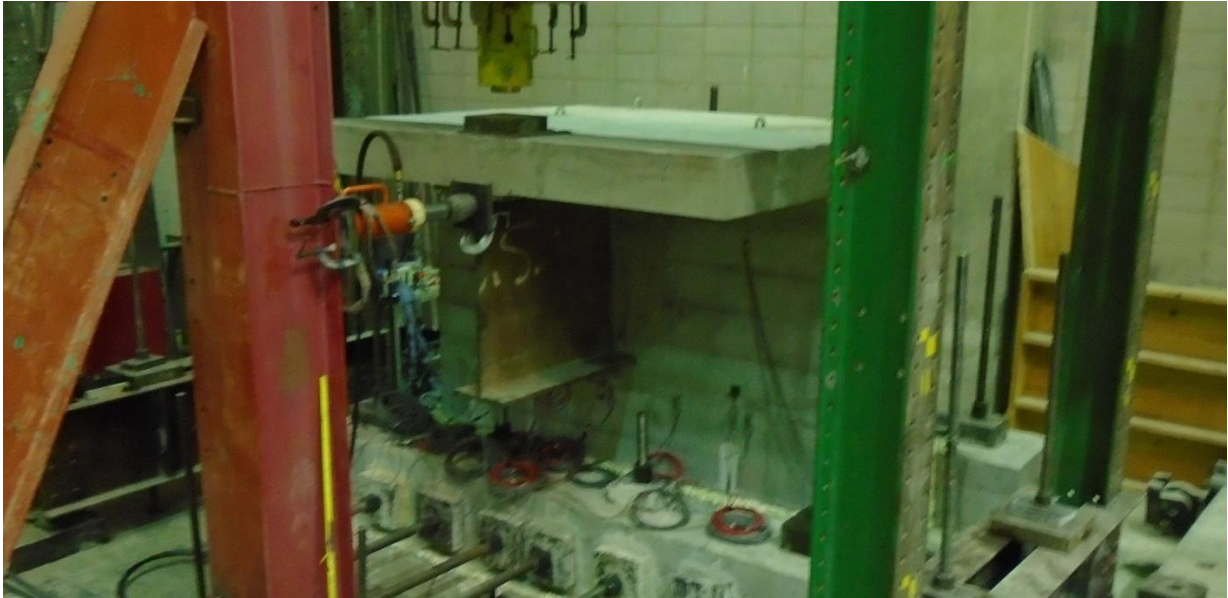
Figure 56. Laboratory loading, horizontal and vertical actuators
