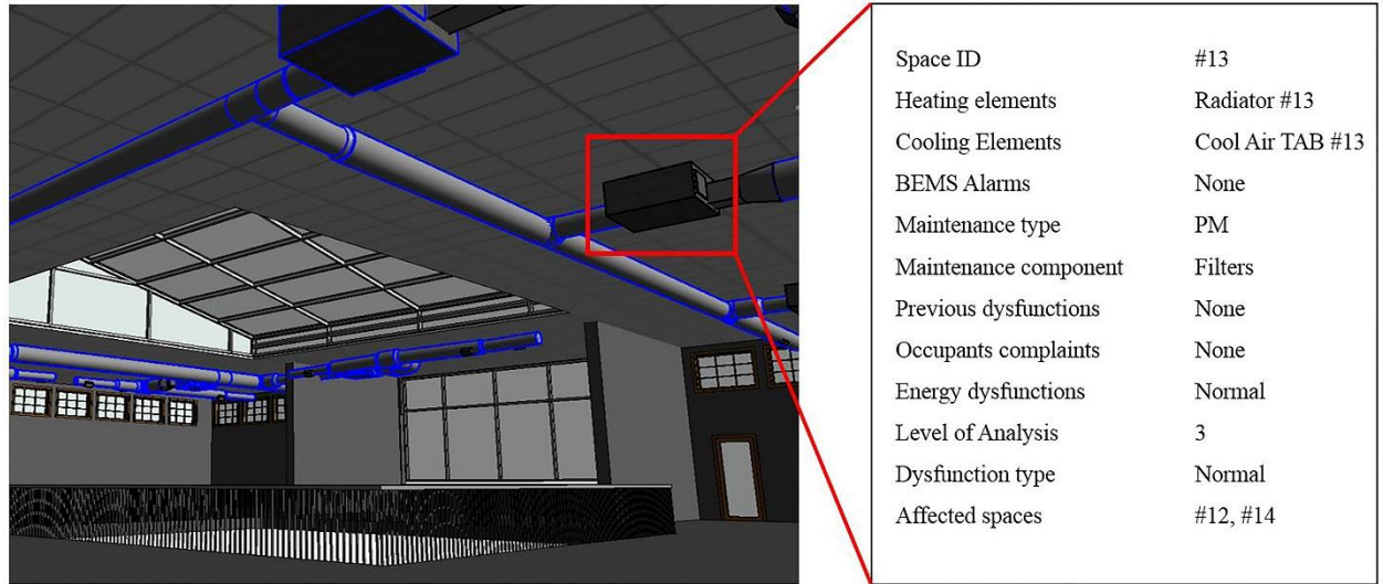
Figure 5.20: BIM framework interface
