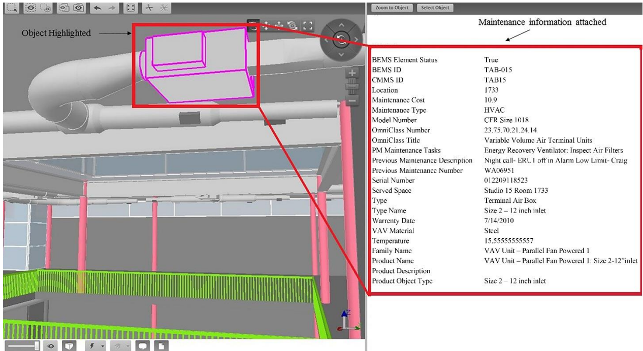
Figure 13: Final IFC-BIM with Maintenance Information
