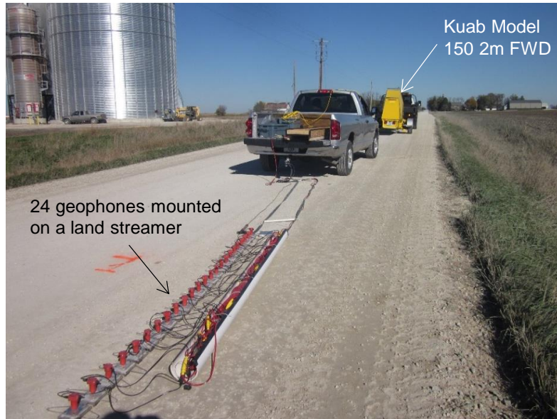
Figure 6.2. FWD and MASW testing setup.
