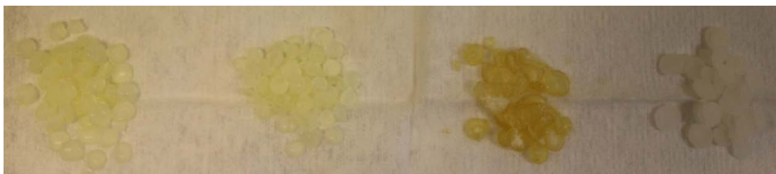
Figure 7 Tackifiers, left to right: Piccotac 1095, Piccotac 8095, Staybelite 10-E, Foral AX-E
