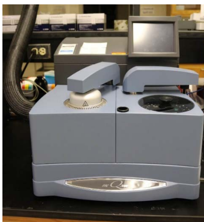
Figure 17 Differential Scanning Calorimetry (DSC) apparatus
