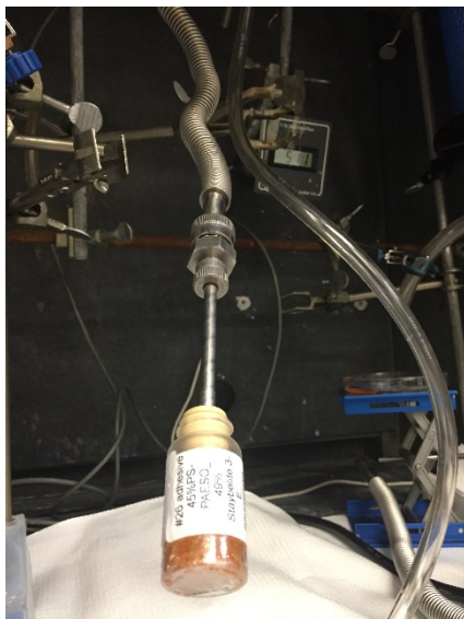
Figure 13 Drying of the PSA with schlenkline setup
