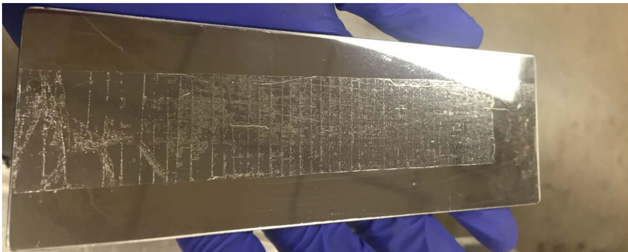
Figure 37 Peeling the PSA film containing Staybelite 10-E
