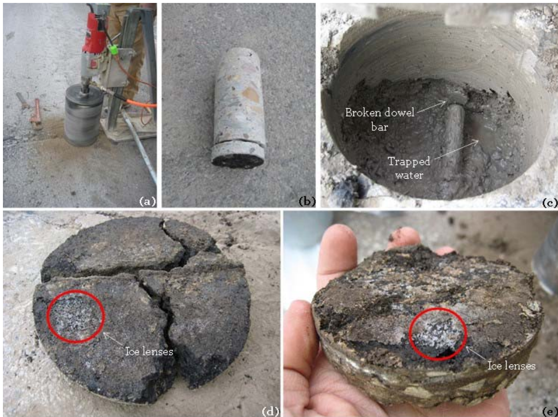
Figure 4.2. Core extraction and inspection: (a) drilling core from pavement surface, (b) subsurface concrete specimen, (c) holes with trapped water, (d) broken asphalt concrete specimen, and (e) presented ice lenses.
