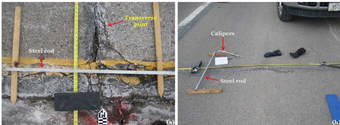
Figure 4.3. Measuring vertical heaves at transvers joint locations.
